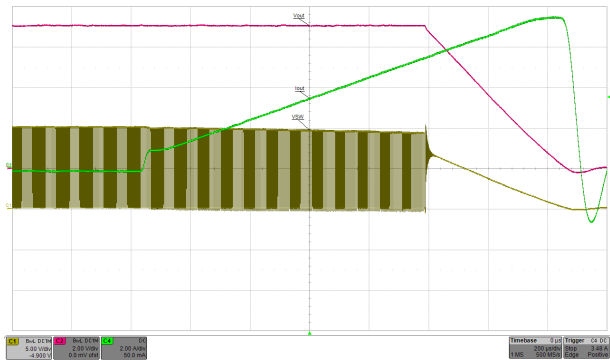
10Vin, 7.0Vout, excessive 10A load applied, OCP=5.6A
