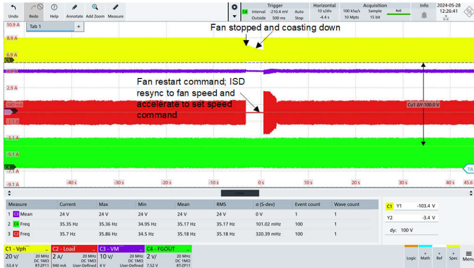
Figure 4-6. Forward Windmilling (High Speed ISD Forward Resync)
