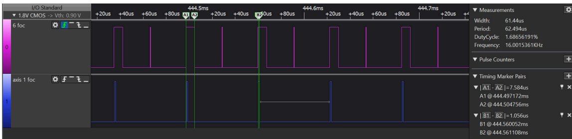
Figure 4-18. 6-Axis FOC Loop Processing Time
