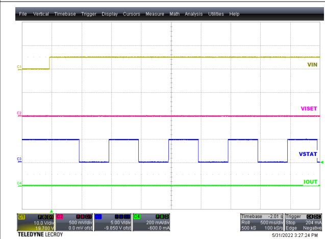
Figure 8-7. Input OVP Response
