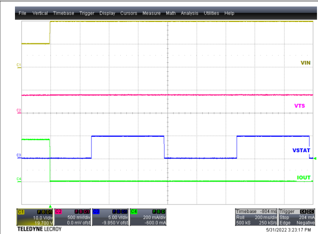
Figure 8-7. Input OVP Response
