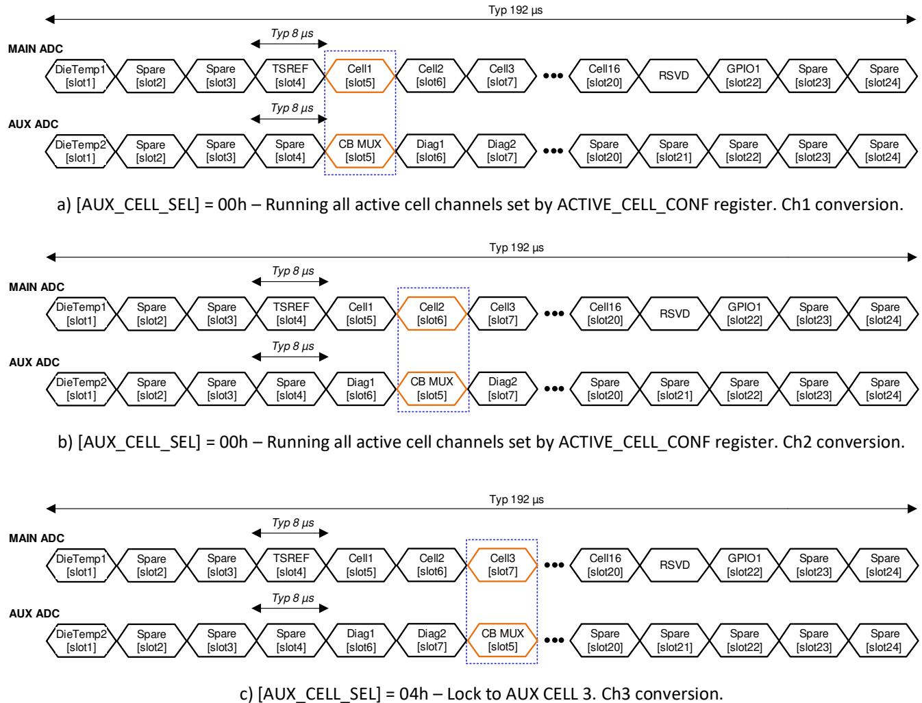
Figure 8-11. Synchronization between MAIN and AUX ADC Sampling
