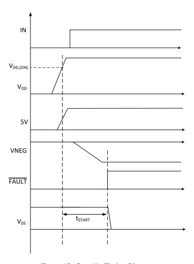
Figure 15. Start Up Timing Diagram
