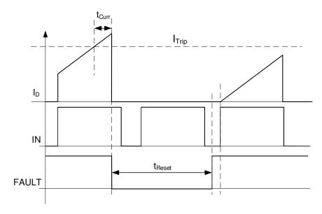
Figure 17. OC Latching and Reset Sequence
