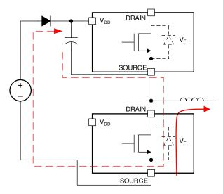
Figure 21. Charging Path for Bootstrap Diode
