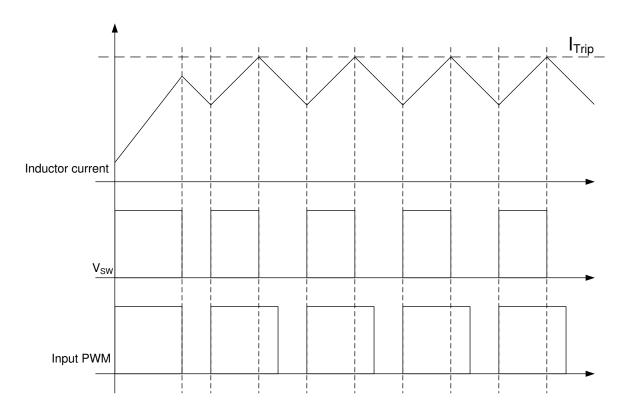
Figure 18. Cycle-by-cycle OCP Operation
