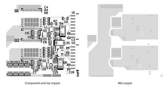
Figure 23. Example Half-Bridge Layout
