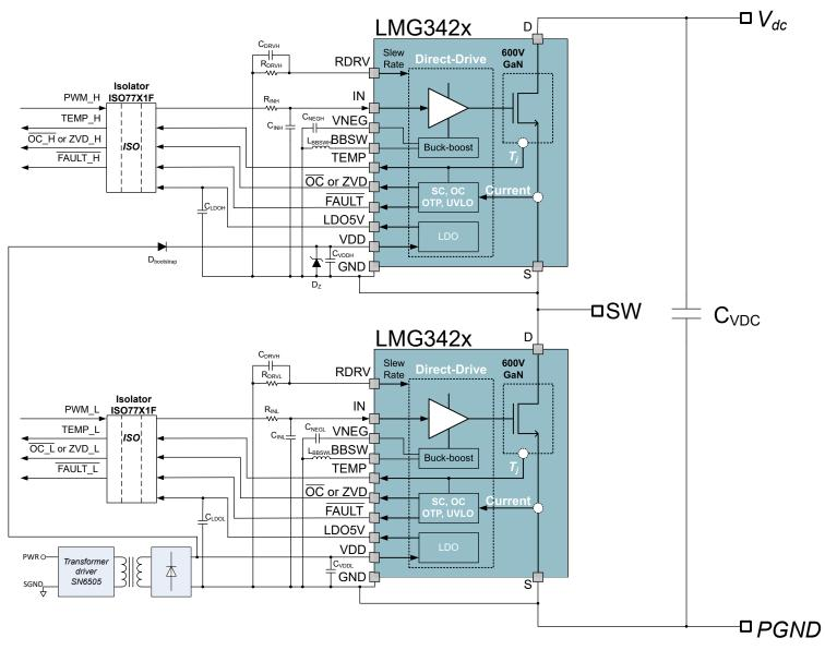
Figure 8-2. Typical Half-Bridge Application With Bootstrap
