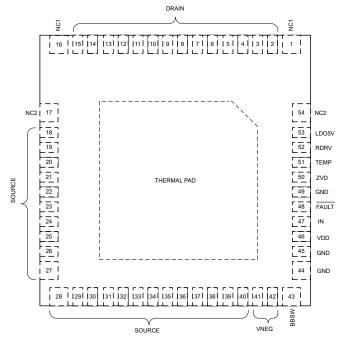
Figure 4-2. LMG3426R050 RQZ Package, 54-Pin VQFN (Top View)
