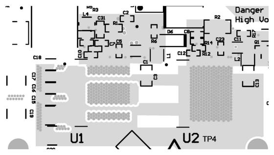
Figure 8-11. Half-Bridge Mid-Layer Layout
