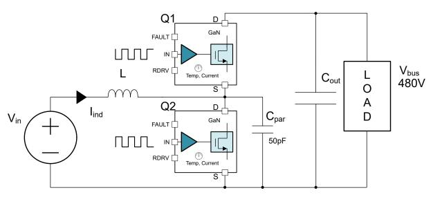
Figure 6-4. Circuit Used for SOA Curve
