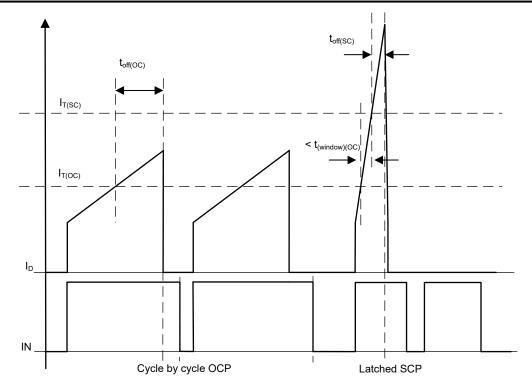
Figure 7-5. Overcurrent Detection vs Short-Circuit Detection
