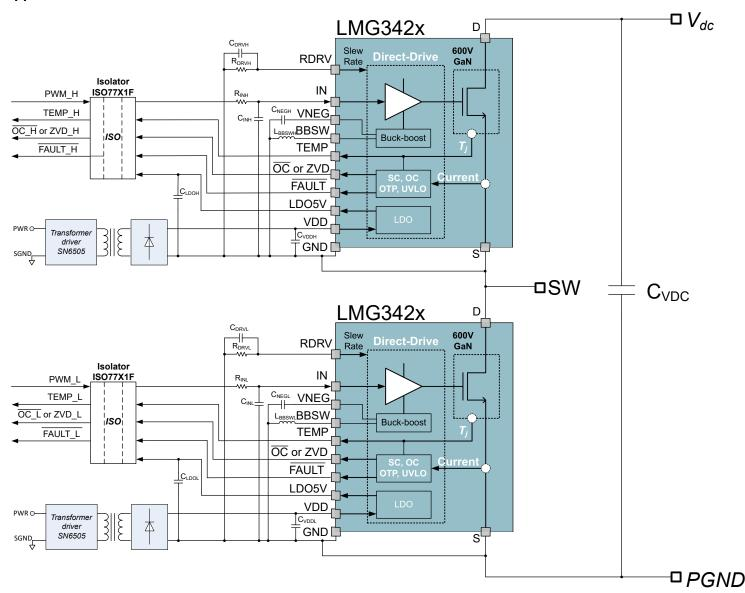
Figure 8-1. Typical Half-Bridge Application With Isolated Power Supply
