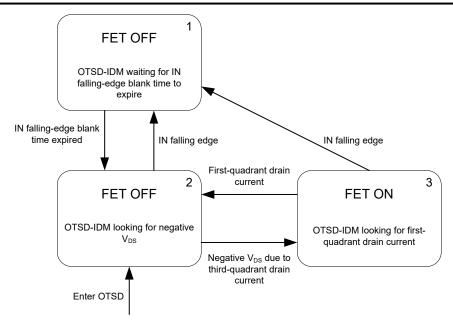
Figure 7-6. Overtemperature-Shutdown Ideal-Diode Mode (OTSD-IDM) State Machine
