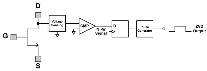
Figure 7-7. Circuit Diagram for Zero-Voltage Detection Circuit Block Diagram
