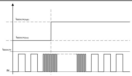
Figure 7-3. Buck-Boost Converter Peak Current
