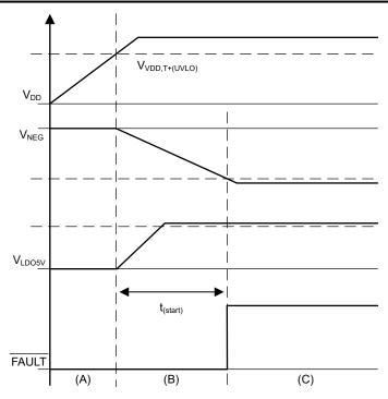
Figure 7-10. Start-Up Timing Diagram
