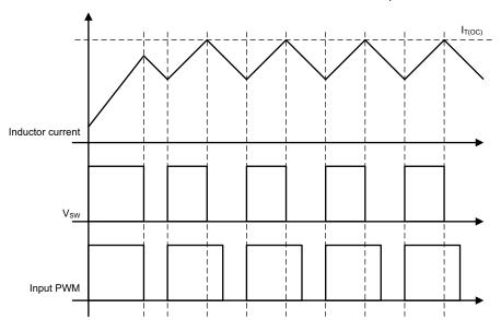
Figure 7-4. Cycle-by-Cycle OCP Operation
