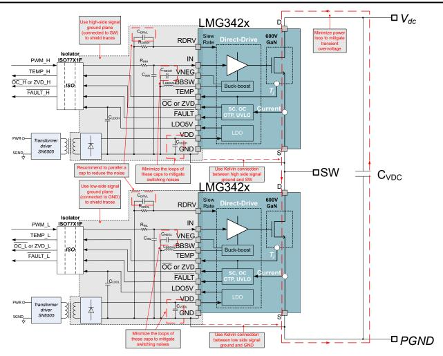
Figure 8-9. Typical Schematic With Layout Considerations
