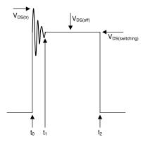
Figure 7-1. Drain-Source Voltage Switching Cycle
