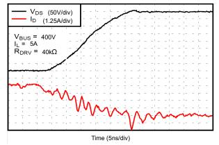
Figure 8-6. Turn-Off Waveform in Application Example
