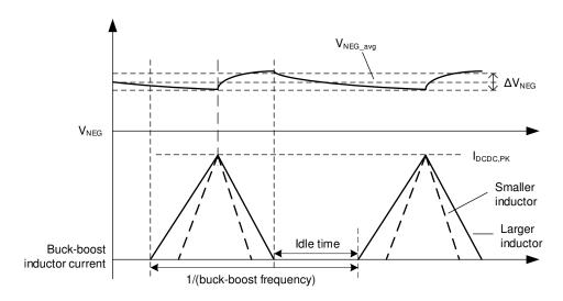
Figure 7-2. Buck-Boost Converter Inductor Current
