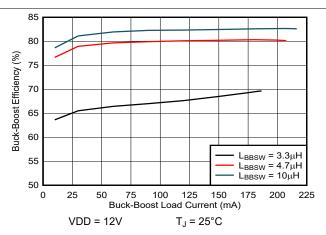
Figure 8-4. Buck-Boost Efficiency vs Load When I<sub>BBSW,PK</sub> = I<sub>BBSW,PK(high)</sub>
