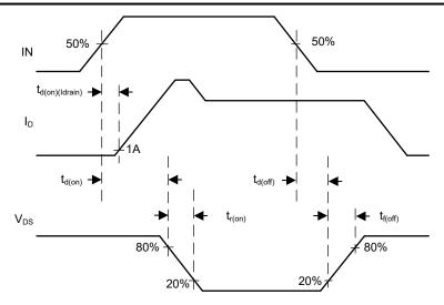
Figure 6-2. Measurement to Determine Propagation Delays and Slew Rates
