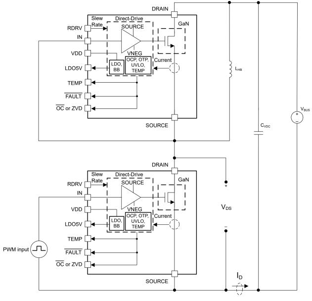
Figure 6-1. Circuit Used to Determine Switching Parameters
