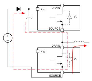
Figure 8-7. Charging Path for Bootstrap Diode
