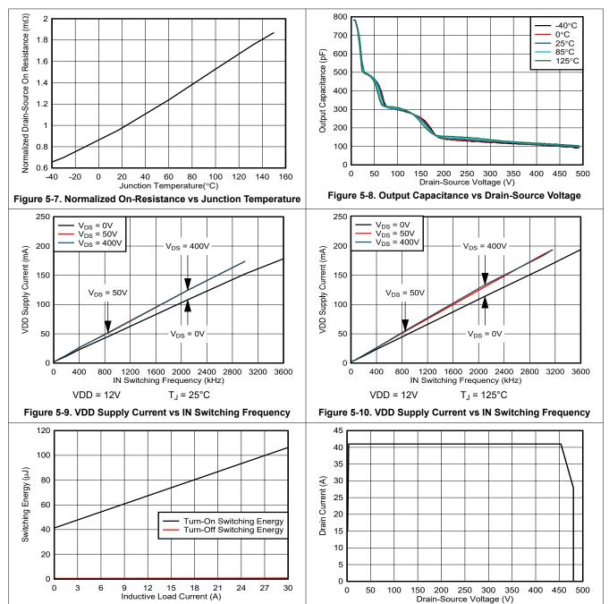
Figure 5-11. Half-Bridge Switching Energy vs Inductive Load
