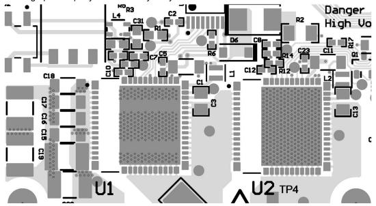
Figure 8-10. Half-Bridge Top-Layer Layout
