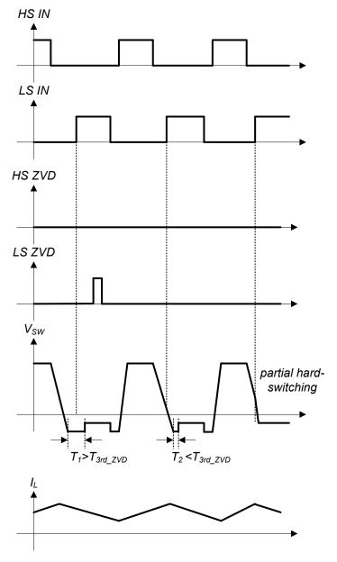
Figure 7-8. ZVD Function in a CCM Buck Converter
