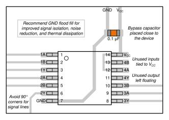
Figure 7-1. Layout Example for the SNx4AC00
