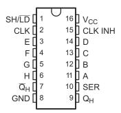
Figure 5-1. D, DB, DGV, N or PW Package, 16-Pin SOIC, SSOP, TVSOP, SOP or TSSOP (Top View)
