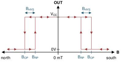
Figure 6-2. Omnipolar Functionality
