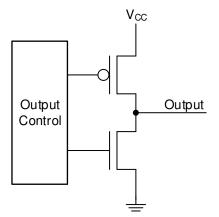
Figure 6-3. Push-Pull Output (Simplified)
