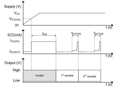
Figure 6-4. TMAG5328A1D Timing Diagram
