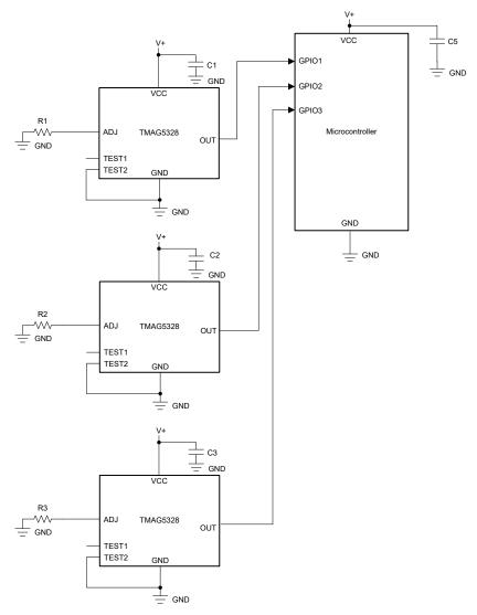
Figure 7-6. Setting B<sub>OP</sub> of Three TMAG5328 Devices Using Three Resistors
