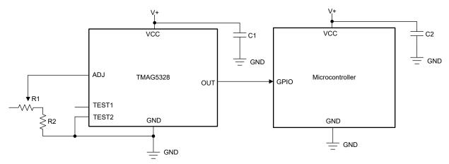
Figure 7-5. Setting B<sub>OP</sub> of One TMAG5328 Device Using a Potentiometer and the TMAG5328's Internal Current Source
