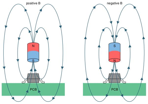
Figure 6-1. Flux Direction Polarity
