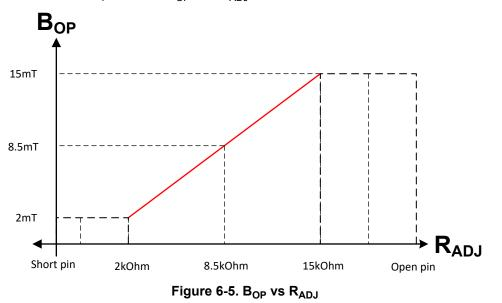
Figure 6-5 shows the relationship between B<sub>OP</sub> and R<sub>ADJ</sub>.
