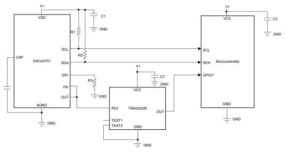
Figure 7-2. Setting B<sub>OP</sub> of One TMAG5328 Device Using a DAC
