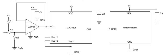
Figure 7-4. Setting B<sub>OP</sub> of One TMAG5328 Device Using a Voltage Divider and Potentiometer
