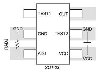
Figure 7-9. SOT-23 Layout Example
