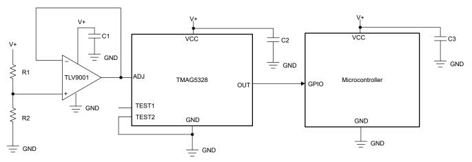
Figure 7-3. Setting B<sub>OP</sub> of One TMAG5328 Device Using a Voltage Divider
