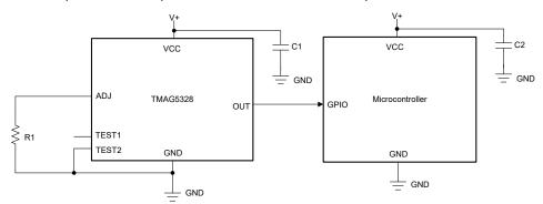
Figure 7-1. Setting B<sub>OP</sub> of One TMAG5328 Device Using a Resistor
