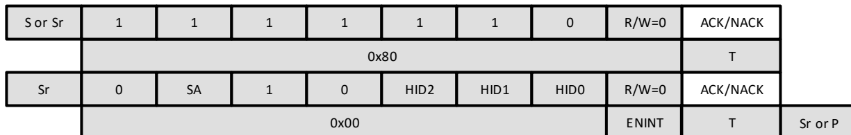
Figure 7-26. ENEC CCC Direct
