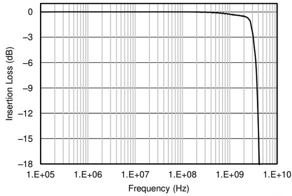
**Figure 6-9. Insertion Loss**
