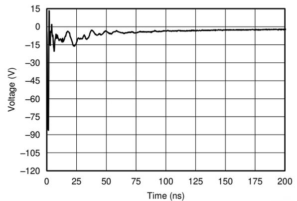
**Figure 6-4. IEC 61000-4-2 Clamping Voltage, -8-kV Contact**
