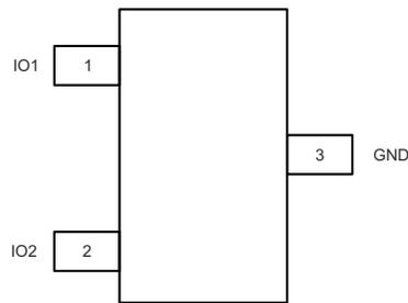
**Figure 5-2. DCK Package, 3-Pin SC70 (Top View)**
