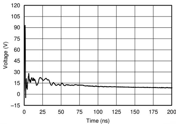
**Figure 6-3. IEC 61000-4-2 Clamping Voltage, 8-kV Contact**
