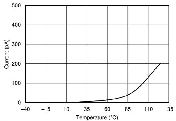
**Figure 6-6.  $I_{LEAK}$  vs Temperature,  $V_{IN} = 2.5\text{ V}$**
