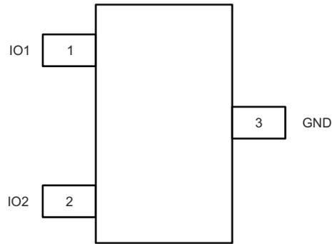
**Figure 5-1. DBZ Package, 3-Pin SOT23 (Top View)**
