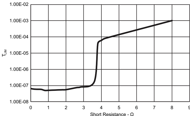
Figure 8. Overcurrent Response Time vs Short Resistance
