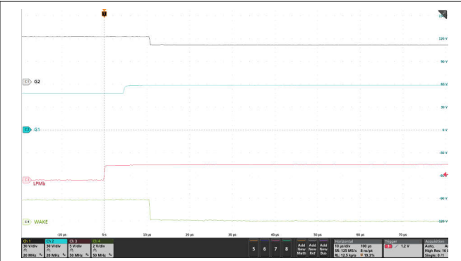
Figure 8-5. State Transition From LPM to Active Mode ( \overline{\text{LPM}} = \text{Low to High} , V_{\text{IN}} = 48\text{V} , No Load)
