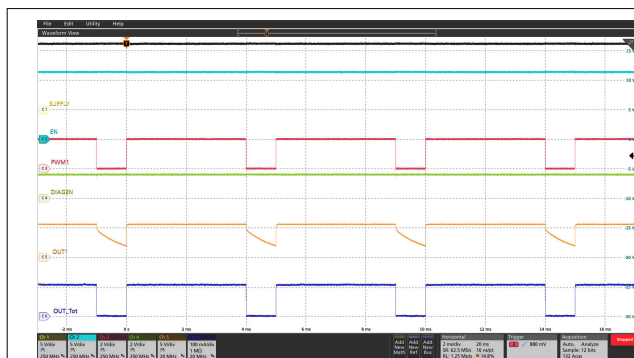
Figure 8-5. PWM Dimming 80% Dutycycle at 200 Hz
