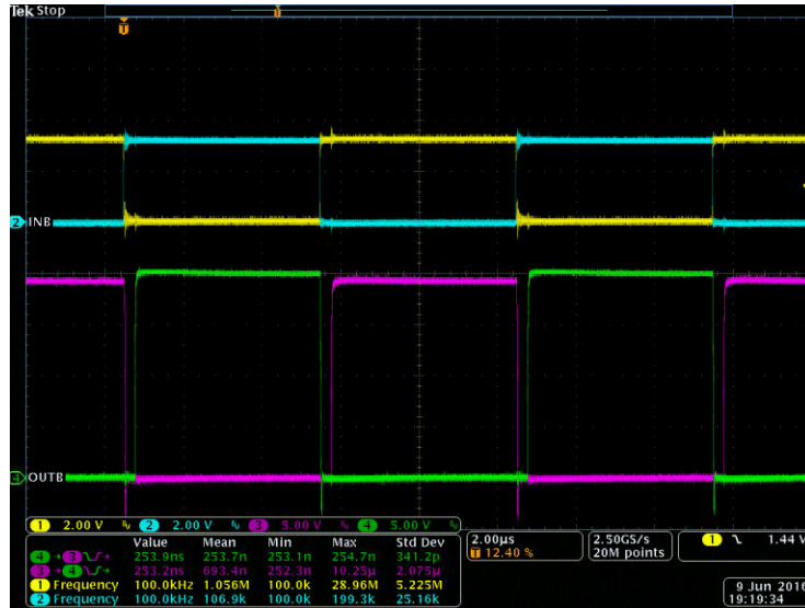
Figure 8-5. Bench Test Waveform for INA/B and OUTA/B
