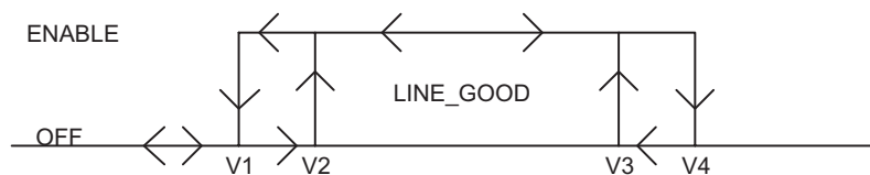
Figure 18. Line UVLO and OVLO Operation
