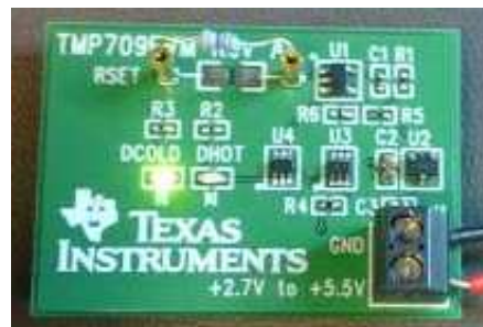
Figure 3. Connecting the Power Supply to the Test Board
