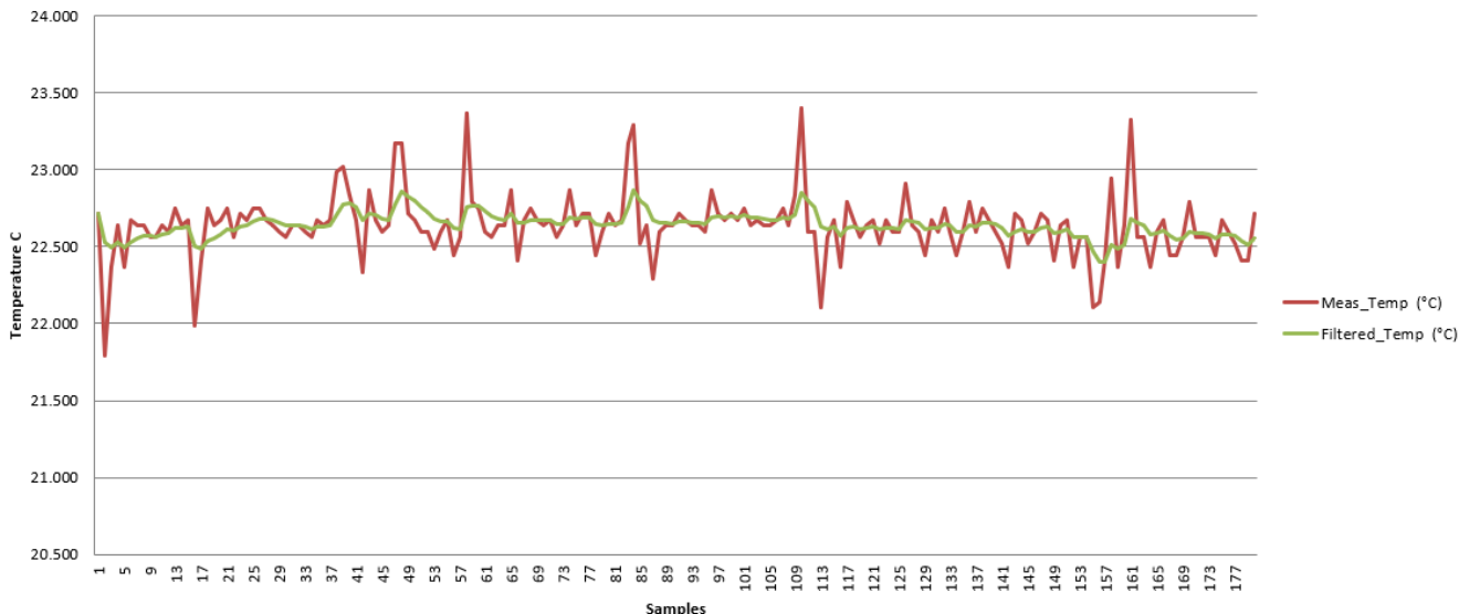
Figure 3-10. Low-Pass Filter Response With 0.2 Alpha Value
