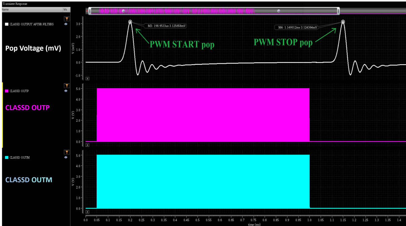
Figure 2-2. Measured Pop Due to Start and Stop of Class-D PWM
