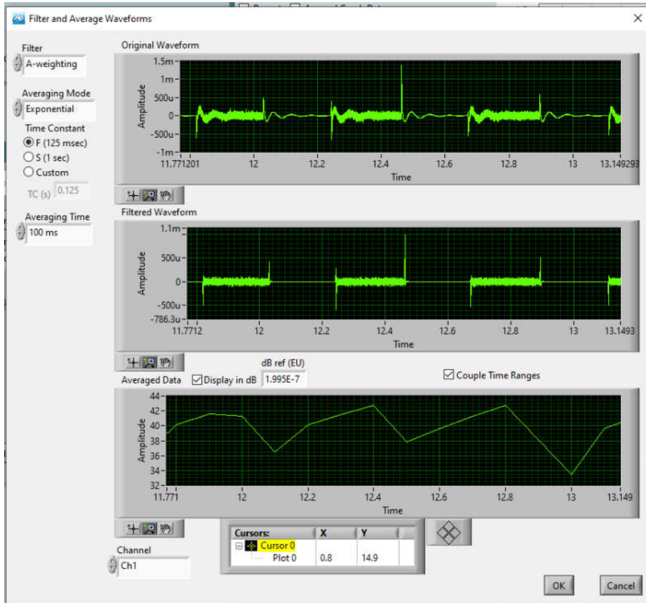
Figure 6-14. Filter and Average Waveform Window – Zoomed Around Max. Peak Level
