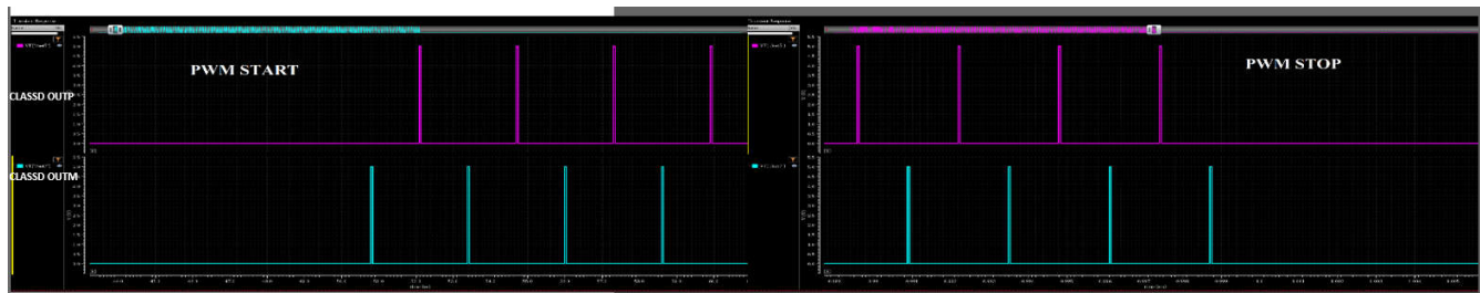
Figure 1-1. Sample LSR Modulated Class-D PWM Output Switching Waveforms at the Start and Stop
