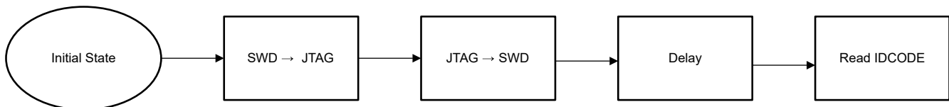
Figure 2-1. MSPM0 SWD Initialization Sequence
