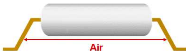
Figure 2. Clearance across a isolator package
