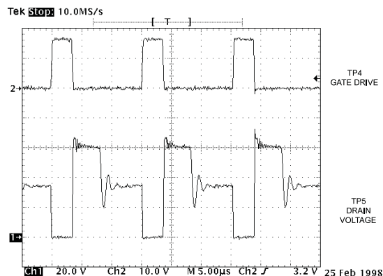
Figure 17. Gate and drain in discontinuous conduction mode.
