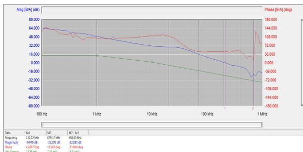
Figure 4-5. Bode Plot at 0.5 V Output Voltage
