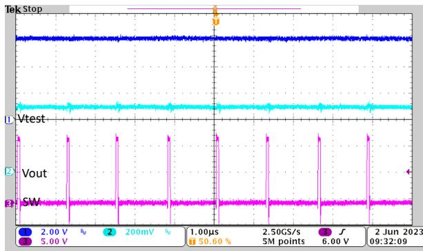
Figure 4-3. Steady State at 0.5 V Output Voltage and 6 V External Test Voltage
