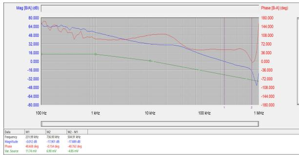
Figure 4-7. Bode Plot at 0.7 V Output Voltage
