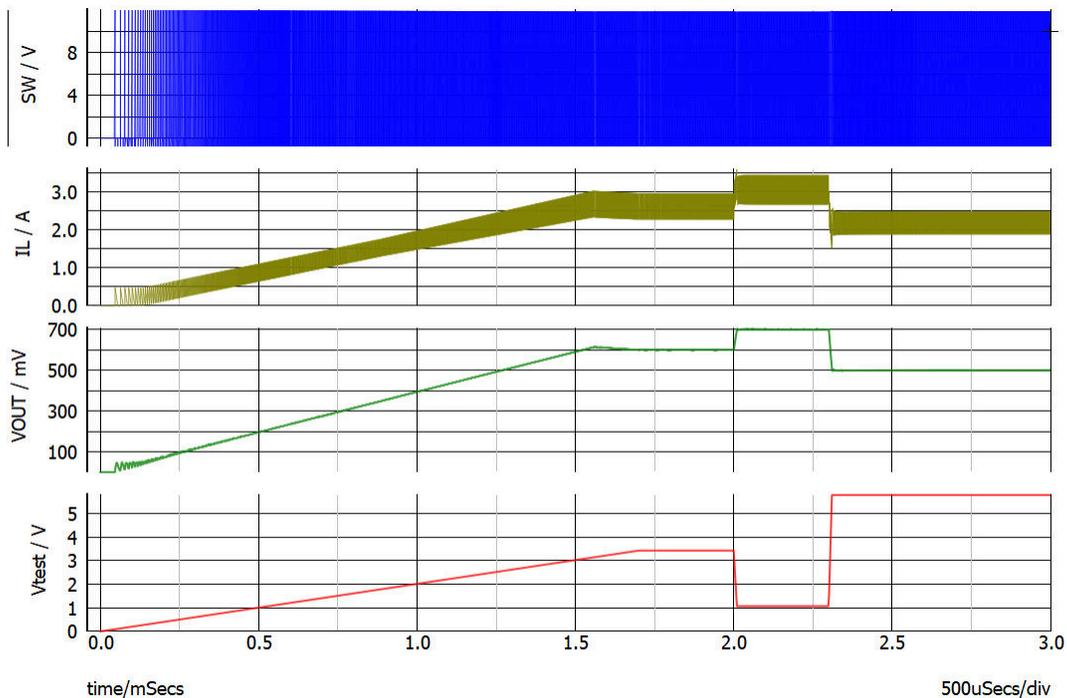
Figure 3-2. Output Voltage Waveform at Different Vtest Voltage
