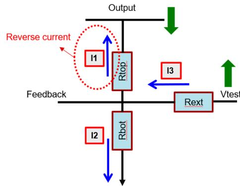
Figure 2-2. Lower Output Voltage With AVS
