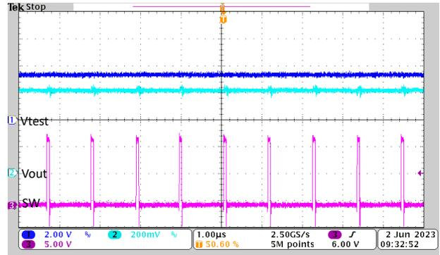
Figure 4-2. Steady State at 0.6 V Output Voltage and 3 V External Test Voltage
