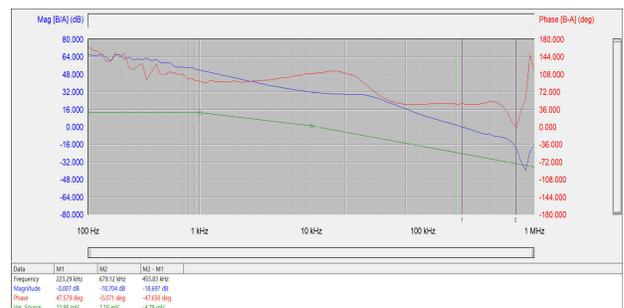
Figure 4-6. Bode Plot at 0.6 V Output Voltage
