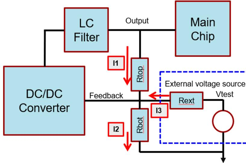
Figure 2-1. Adjustable Output Voltage With AVS
