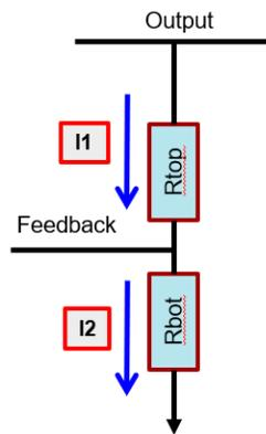
Figure 2-3. Typical FB Circuit
