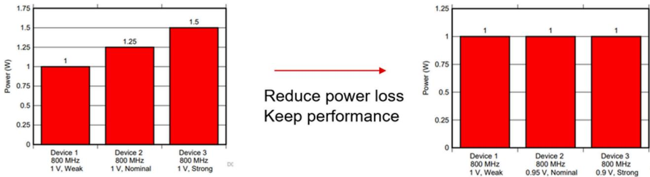
**Figure 1-1. Example of AVS Normalization Effect Across Process Variation**
