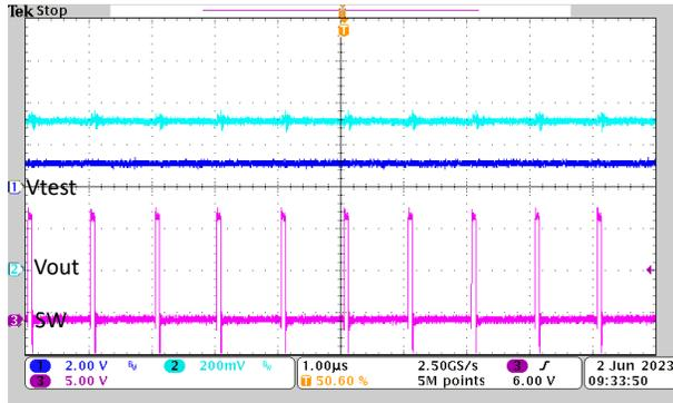
Figure 4-1. Steady State at 0.7 V Output Voltage and 1 V External Test Voltage
