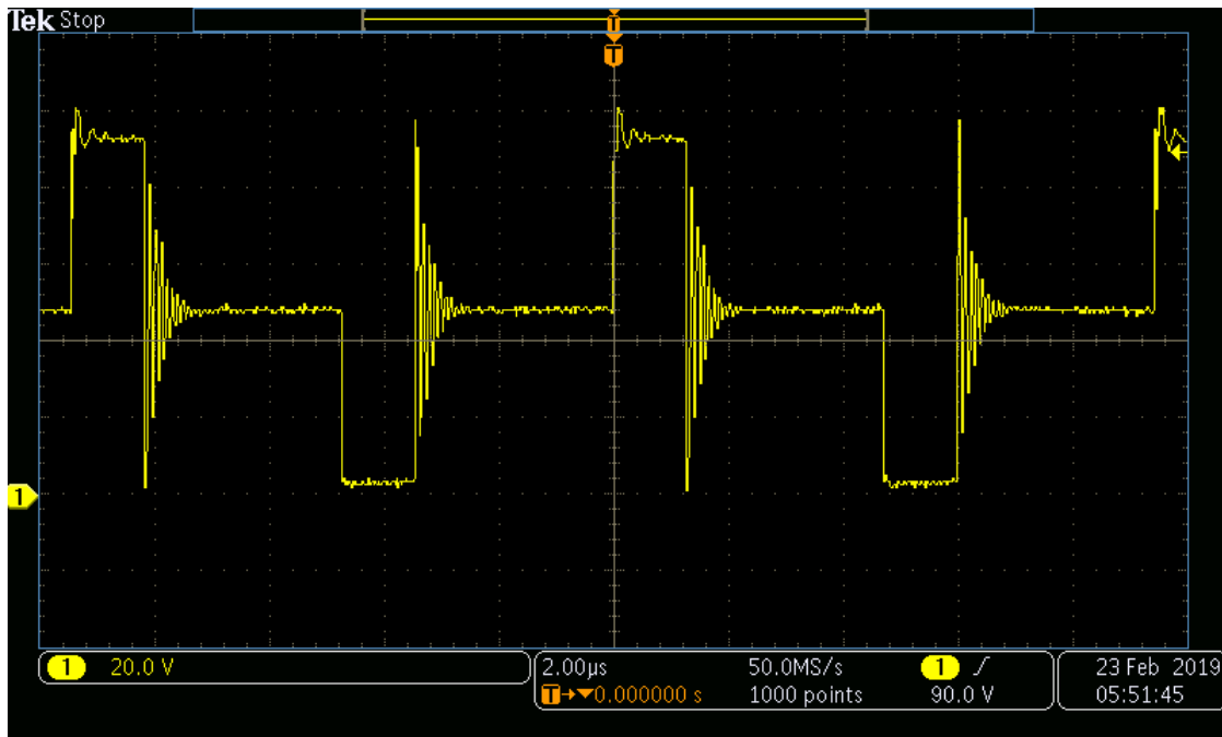
Figure 22. Voltage Stress Across Main Switching MOSFETS Q1 and Q2
