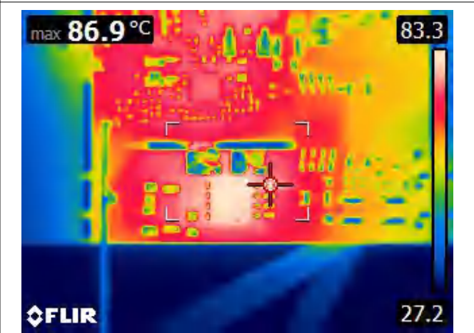
Figure 8-17. V_{IN} = 250 V_{DC} , Bottom-side SR-FET gate-drive R11: 86.9°C
