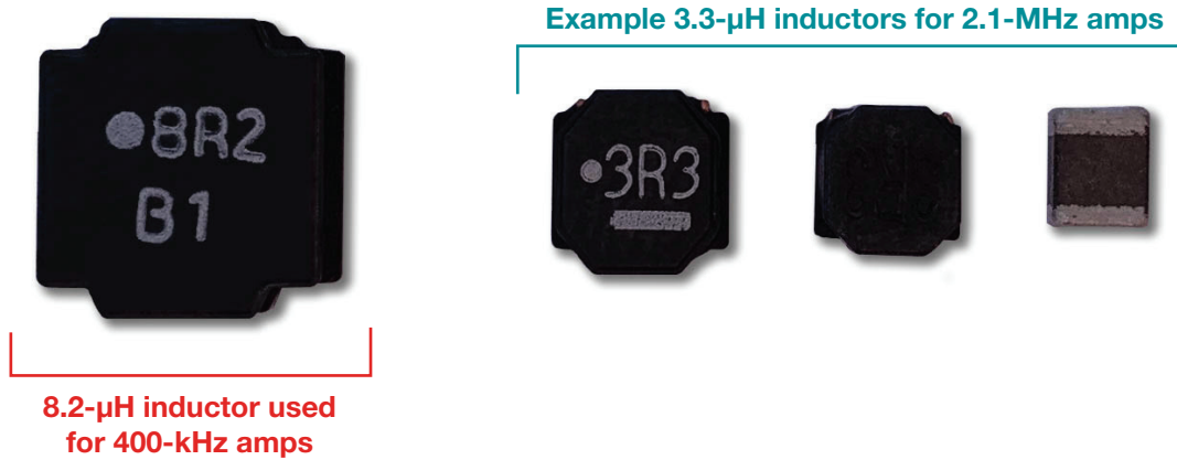
Figure 5. Comparison of inductor size vs. switching frequency.
