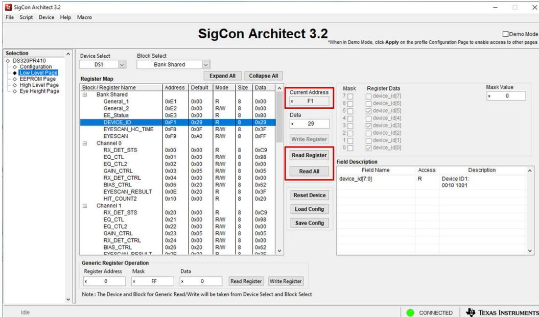
**Figure 3-3. Low Level Page: Read Register Buttons**
