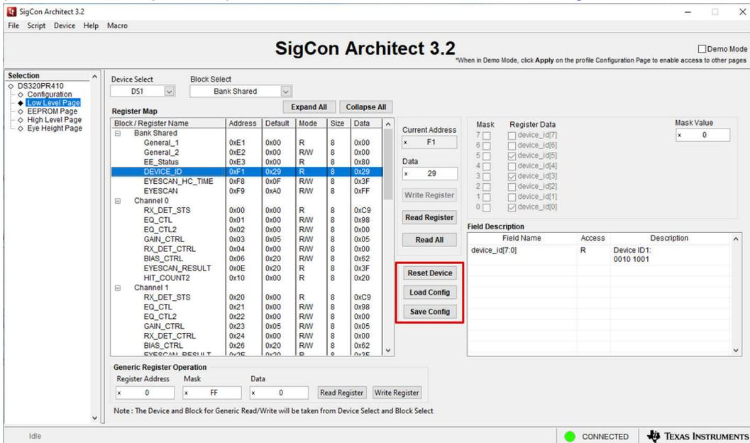
**Figure 3-5. Low Level Page: Reset, Load, and Save Device Configuration Buttons**
