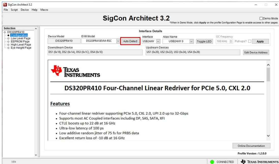
**Figure 2-2. SMBus Address Auto Detect**
