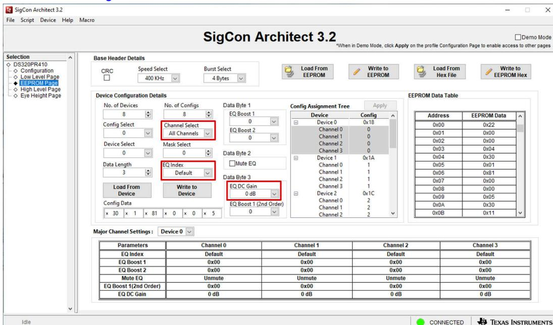
**Figure 4-3. EEPROM Page: Channel Select, EQ Index, and EQ DC Gain**
