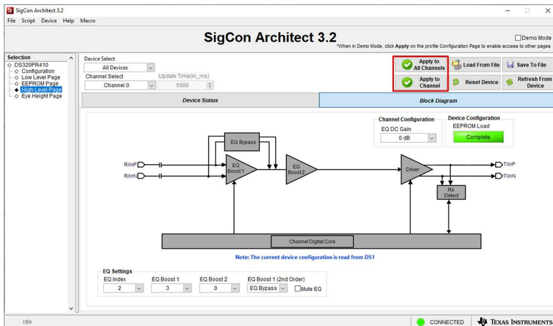
Figure 5-5. High Level Page: Apply to Channel and Apply to All Channels
