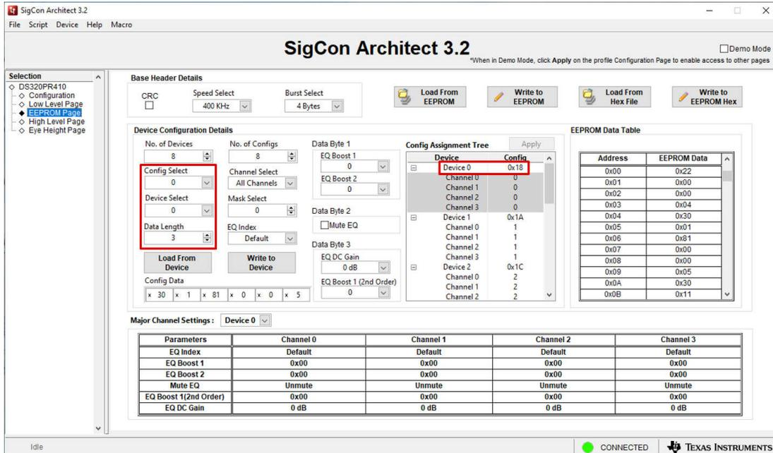
**Figure 4-2. EEPROM Page: Config Select, Device Select, and Configuration Assignment Tree**
