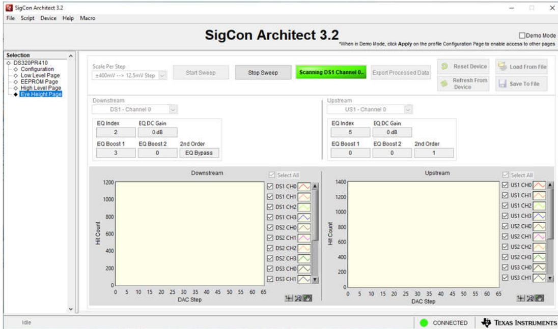
Figure 6-4. Eye Height Page: EyeScan Sweep in Progress
