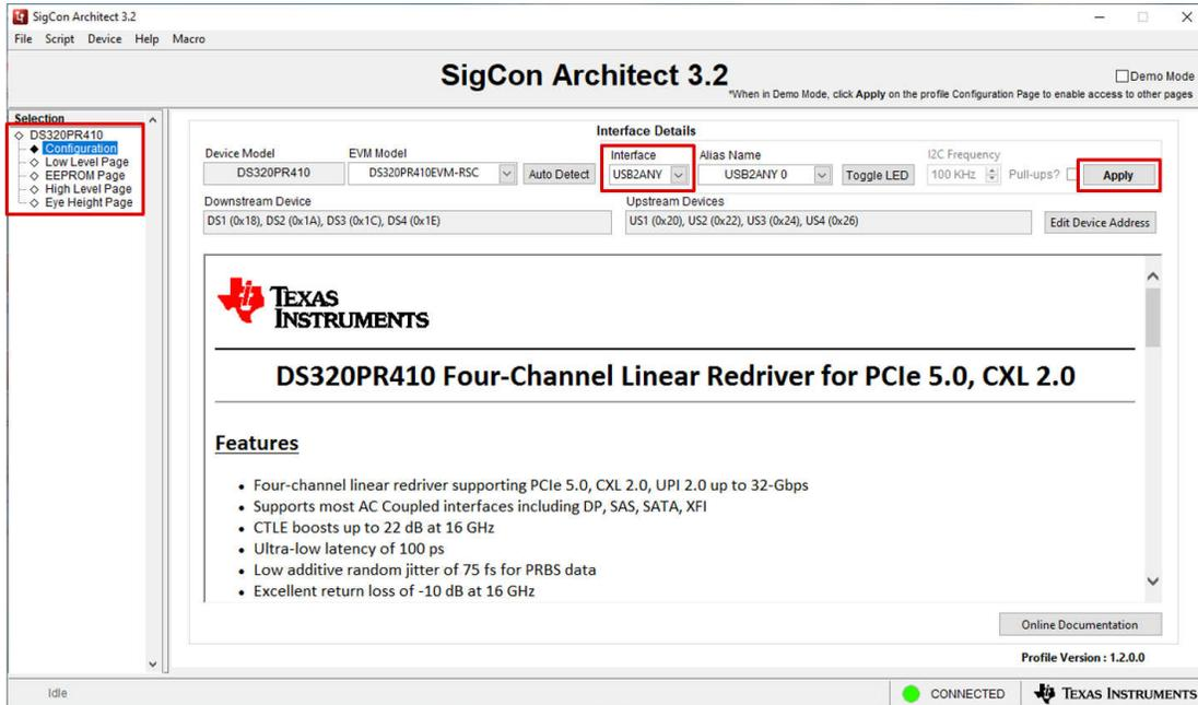
**Figure 2-3. Interface Adapter Select and Apply Settings**
