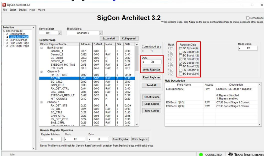
**Figure 3-4. Low Level Page: Data Field and Write Register Button**
