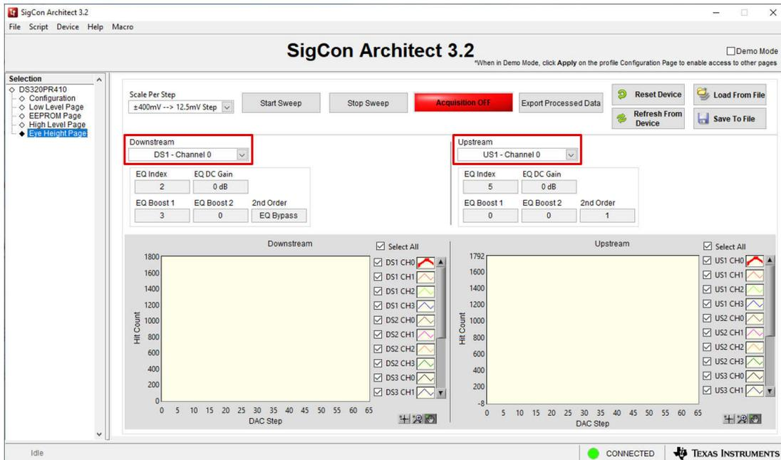
Figure 6-6. Eye Height Page: Plot Channel Selectors
