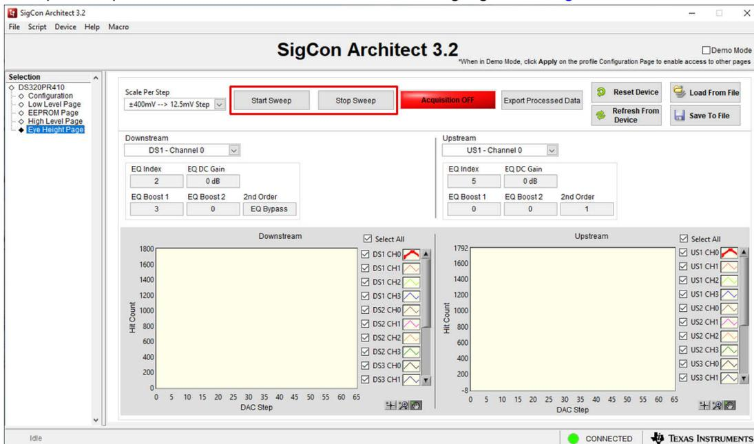
**Figure 6-3. Eye Height Page: Start Sweep and Stop Sweep**
