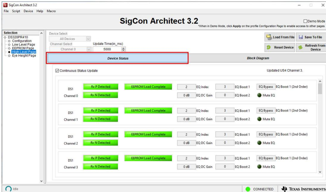
Figure 5-1. High Level Page: Device Status Tab
