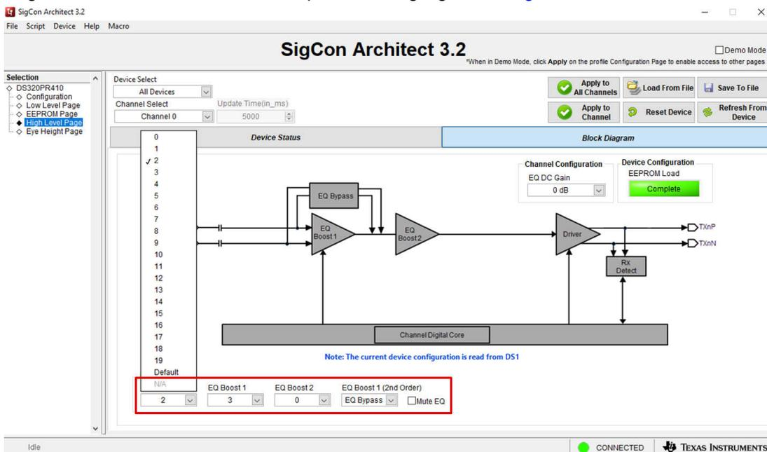
**Figure 5-3. High Level Page: EQ Index and EQ Boost Select**
