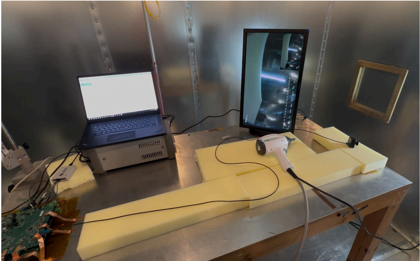
Figure 2-2. ISO 10605 Example Setup
