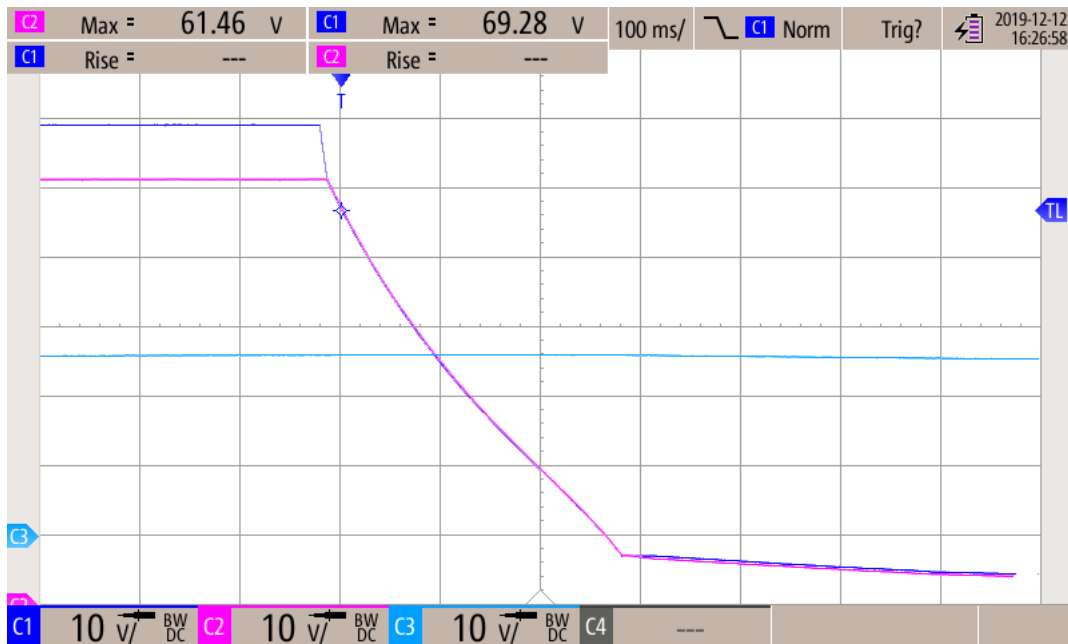
Figure 22. Turn-off Behavior From 70 V to 0 V (No Load)
