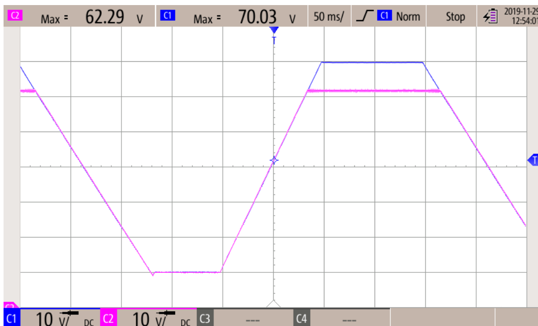
Figure 14. Waveforms for the Circuit with the TL431-Q1 Voltage Regulator (No Load)
