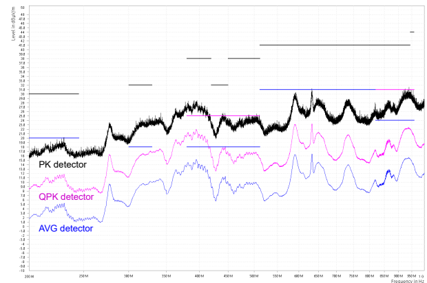
Figure 5-19. CISPR 25 Class 5 Radiated EMI, Log Antenna, Vertical Polarization, 200 MHz to 1 GHz
