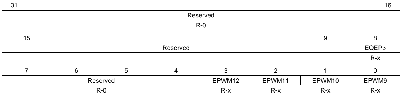
Figure 1-46. Control Subsystem Peripheral Configuration 2 (CCNF2) Register
