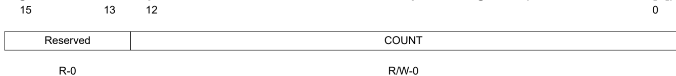
Figure 23-55. USB Request Packet Count in Block Transfer Endpoint n Registers (USBRQPKTCOUNT[ n ])
