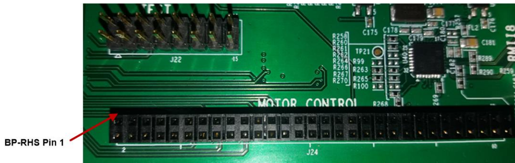
Figure 4-17. Motor Control Header
