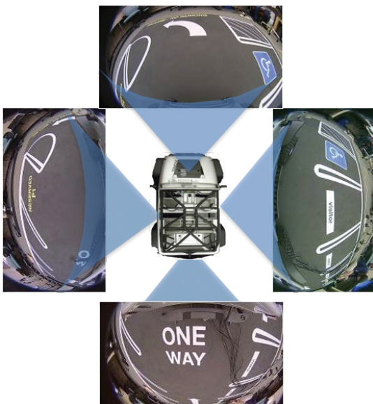
Figure 1: Illustration of a surround view camera system and the fish-eye images captured by each camera.
