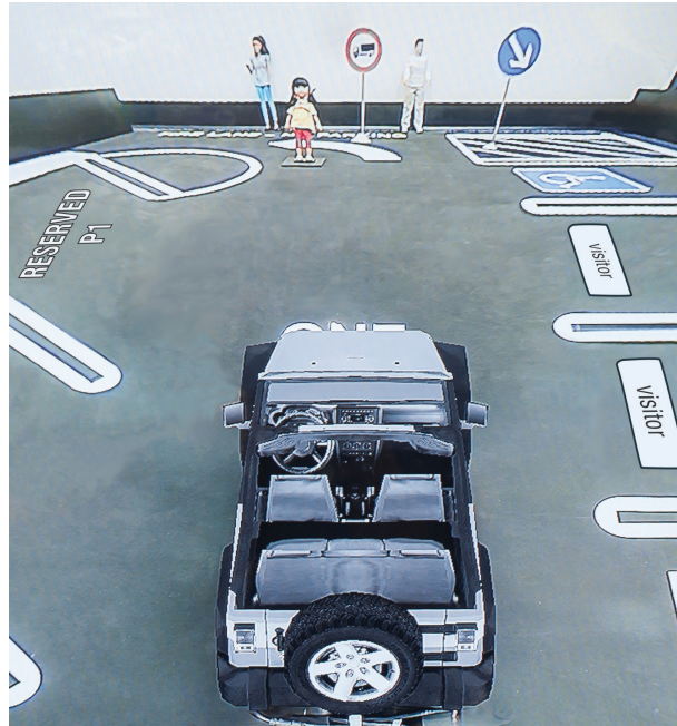
Figure 20: Rendered 3D surround view output of a virtual camera viewpoint of the vehicle from behind.
