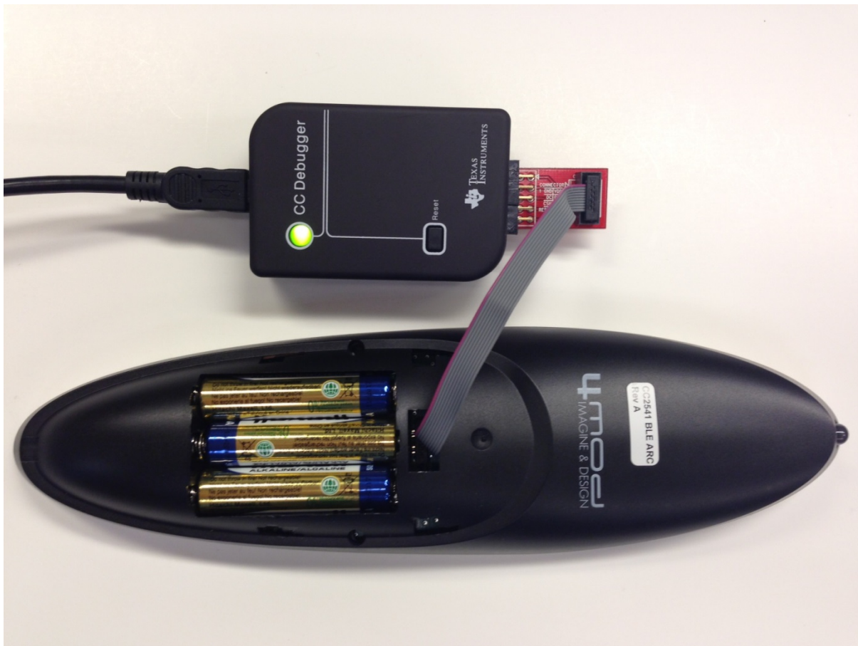
Figure 6-1. Advanced Remote Programming Setup
