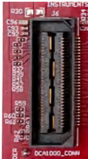
Figure 6-9. DCA1000 HD Connector
