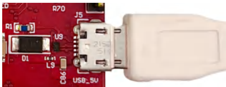
Figure 6-8. USB Connector (J5)
