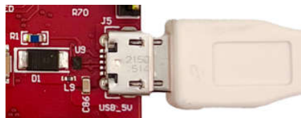
Figure 2-14. USB Connector (J5)
