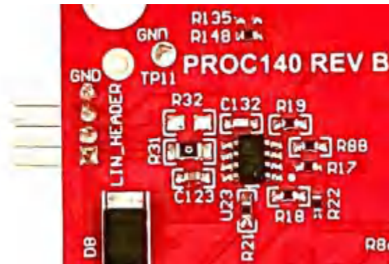
Figure 2-20. LIN header and PHY Interface
