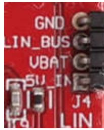
Figure 2-18. LIN header and PHY Interface
