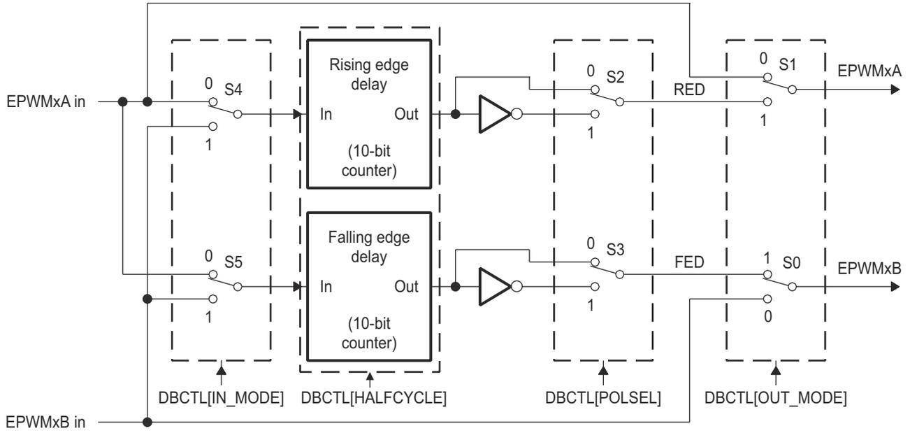
**Figure 18-28. Configuration Options for the Dead-Band Submodule**
