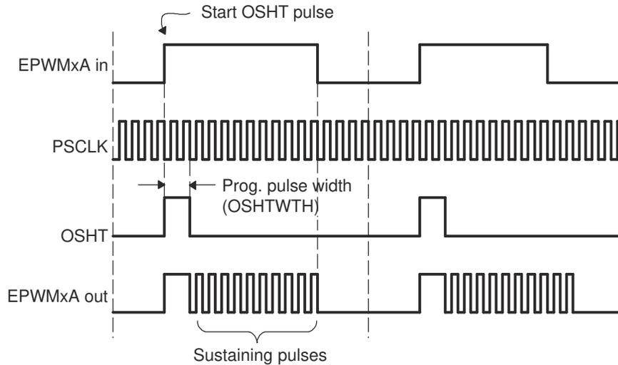
**Figure 18-33. PWM-Chopper Submodule Waveforms Showing the First Pulse and Subsequent Sustaining Pulses**
