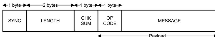
Figure 4-5. Command Packet Format
