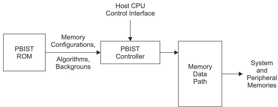
**Figure 22-22. PBIST Block Diagram**
