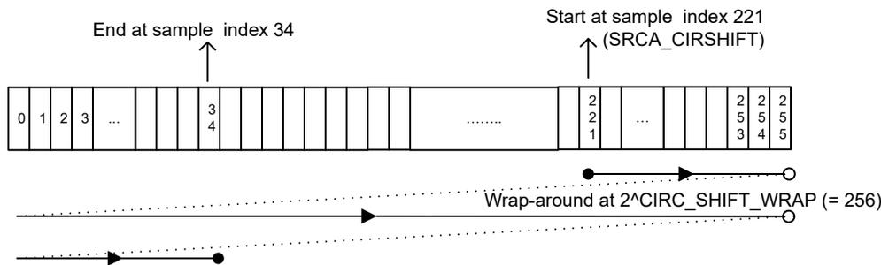
**Figure 10-30. Input Formatter Streaming for Cyclic CFAR example**
