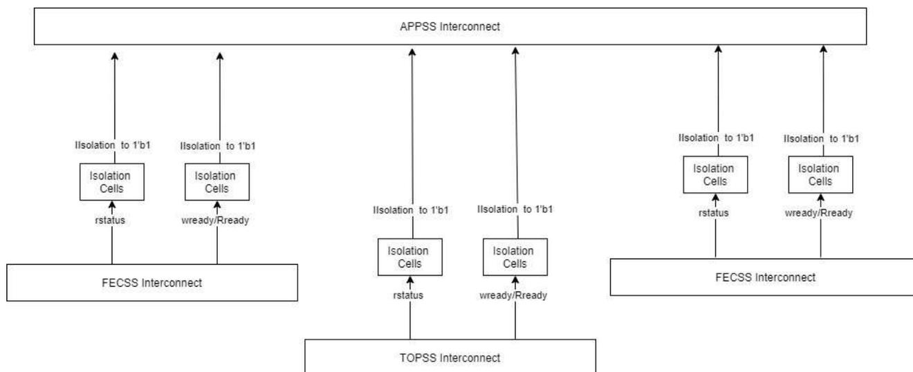
**Figure 22-21. Access Error-Power Domain Accesses**
