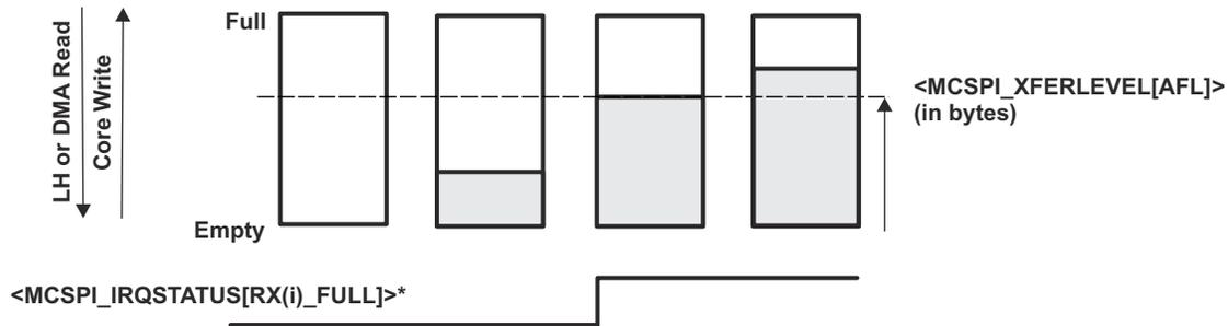
\* non-DMA mode only. In DMA mode, the DMA RX request is asserted to its active level under identical conditions.
