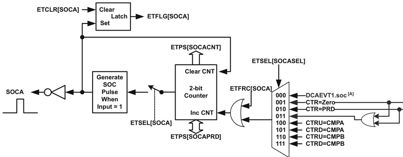
A. The DCAEVT1.soc signals are signals generated by the Digital compare (DC) submodule described later in Section 18.2.9.
