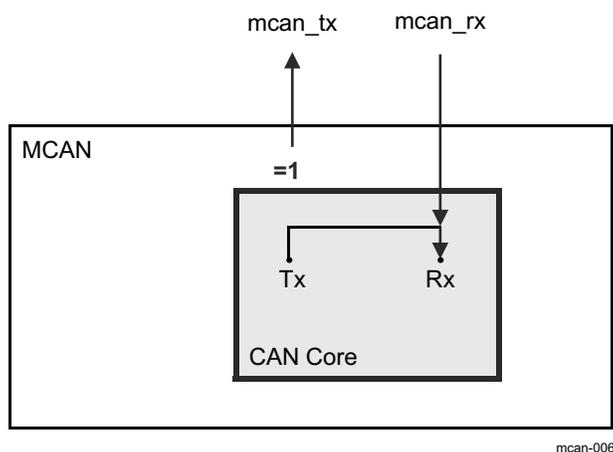
**Figure 12-5. Connection of Signals in Bus Monitoring Mode**
