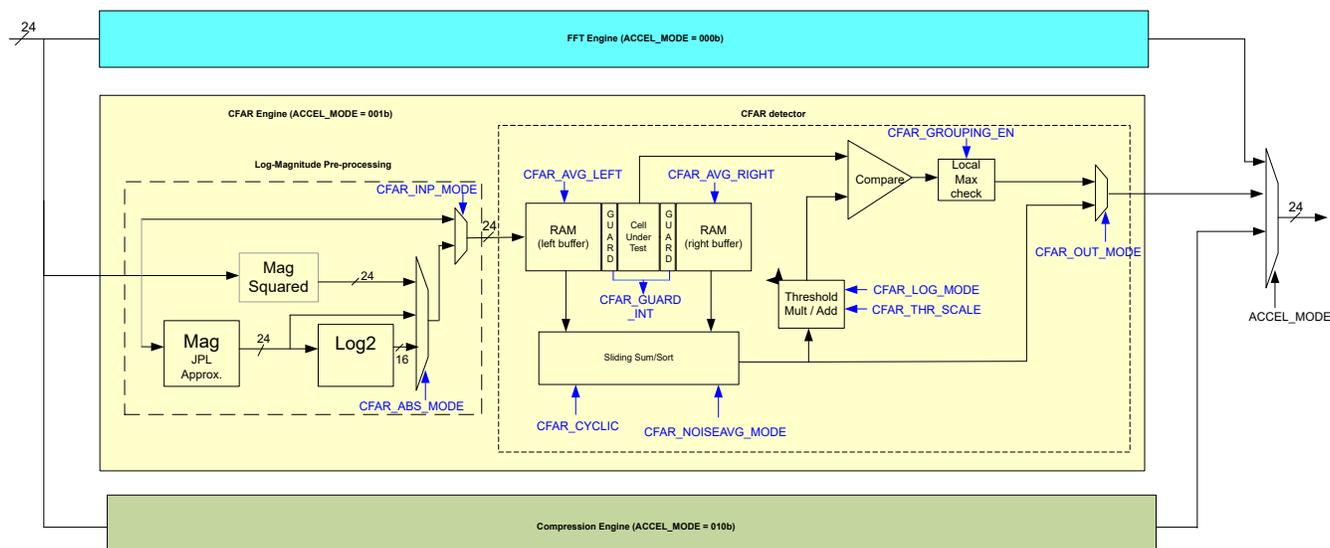
Figure 10-24. CFAR Engine
