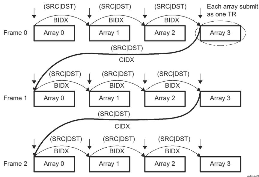
**Figure 11-6. A-Synchronized Transfers (ACNT = n, BCNT = 4, CCNT = 3)**
