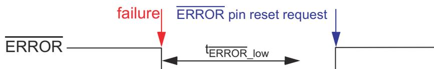
Figure 22-13.  $\overline{\text{ERROR}}$  Pin Timing - Example 3
