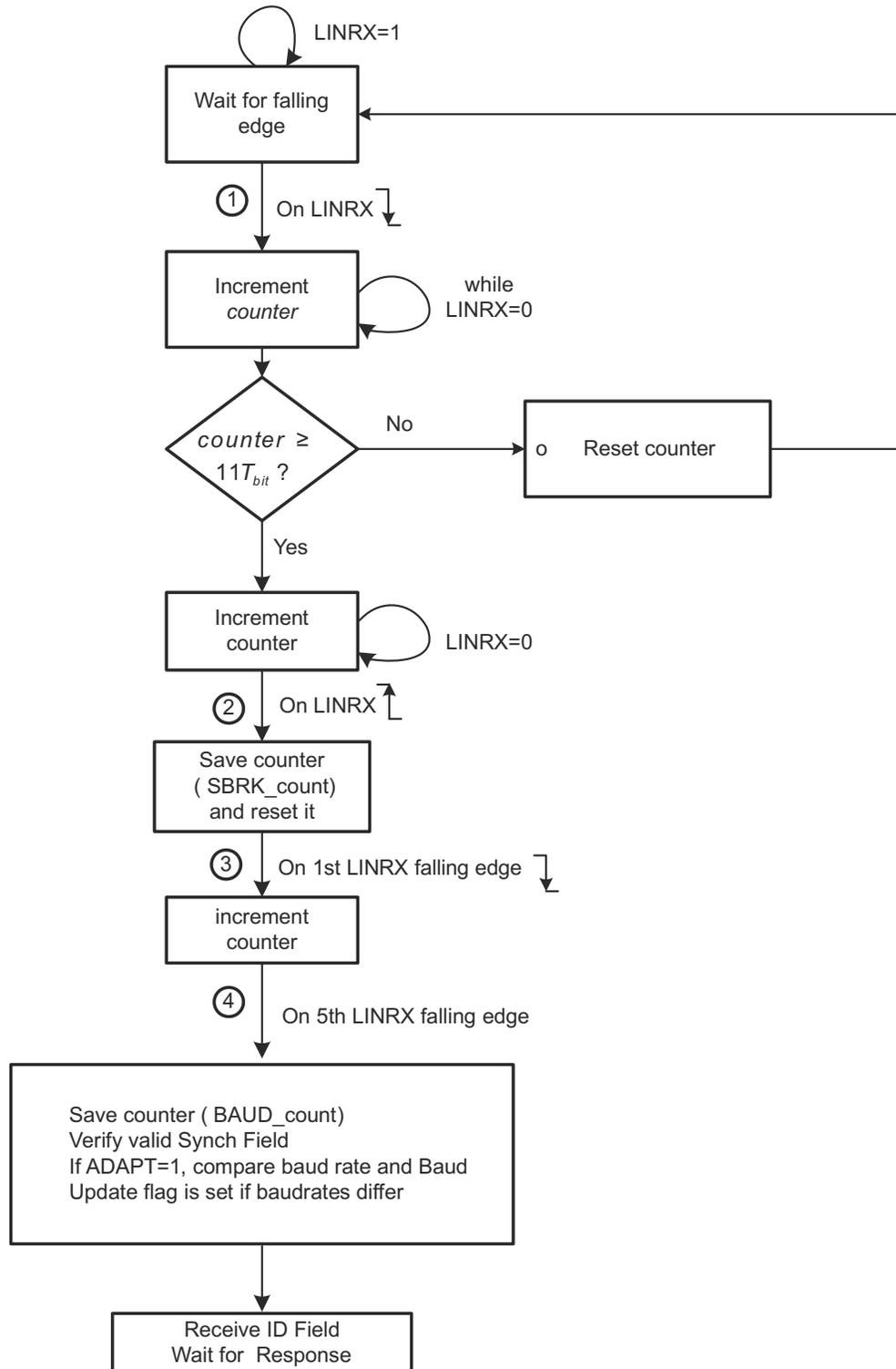
**Figure 19-17. Synchronization Validation Process and Baud Rate Adjustment**
