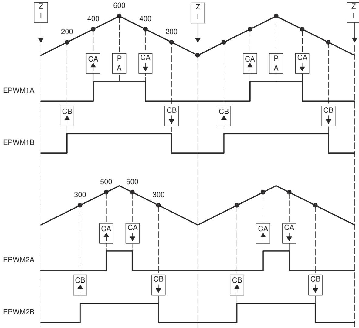
Figure 18-56. Buck Waveforms for Figure 18-55 (Note:  $F_{PWM2} = F_{PWM1}$ )
