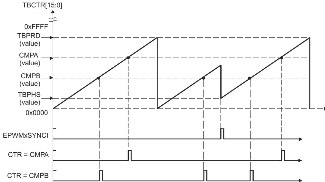
An EPWMxSYNCI external synchronization event can cause a discontinuity in the TBCTR count sequence. This can lead to a compare event being skipped. This skipping is considered normal operation and must be taken into account.
