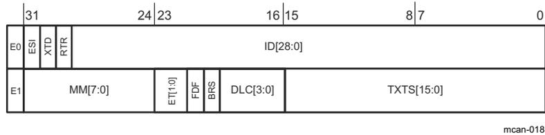
**Figure 12-17. Tx Event FIFO Element Structure**
