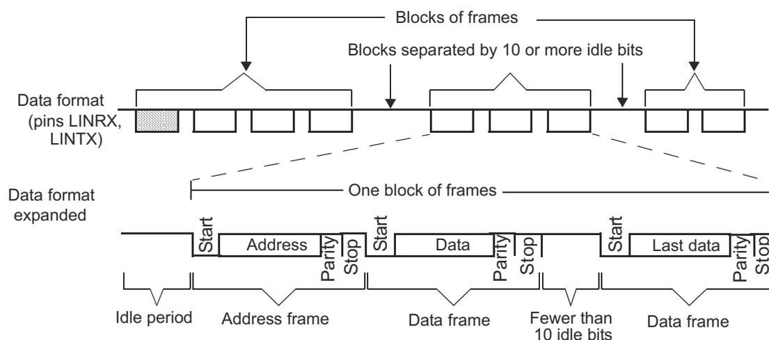
**Figure 19-5. Idle-Line Multiprocessor Communication Format**
