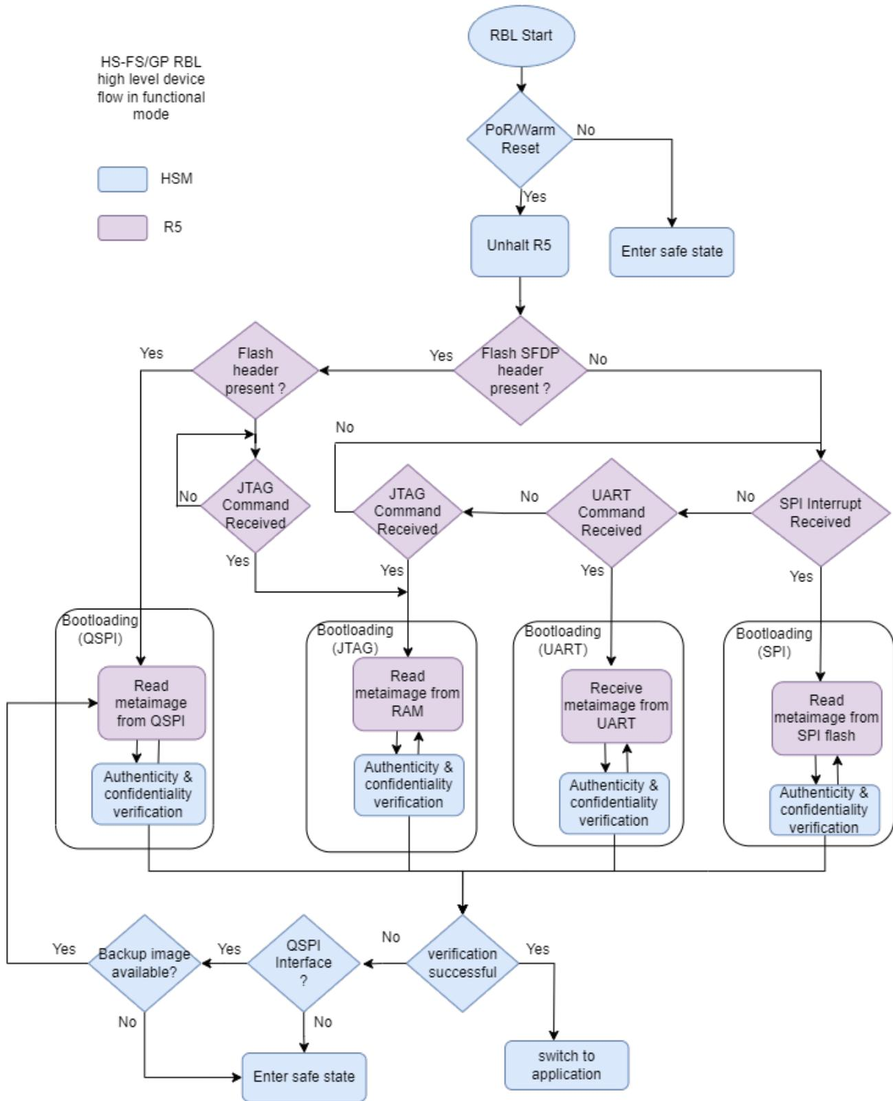
Figure 4-2. High Level Bootloader Flow in Functional Mode
