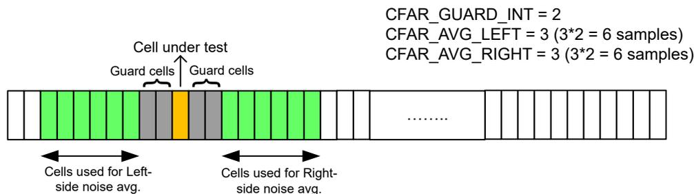
Figure 10-27. CFAR Engine Output Format
