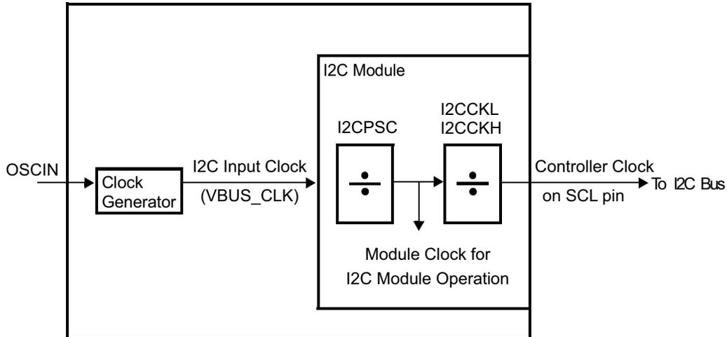
Figure 16-3. Clocking Diagram for the I2C Module
