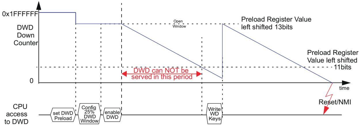
Figure 14-7. Digital Windowed Watchdog Operation Example (25% Window)
