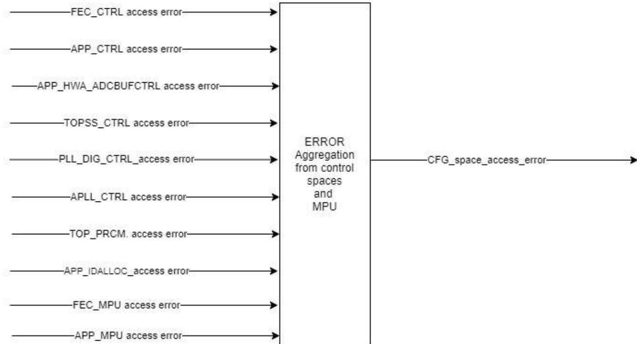
**Figure 22-19. Access Error-CFG\_space\_access\_err**
