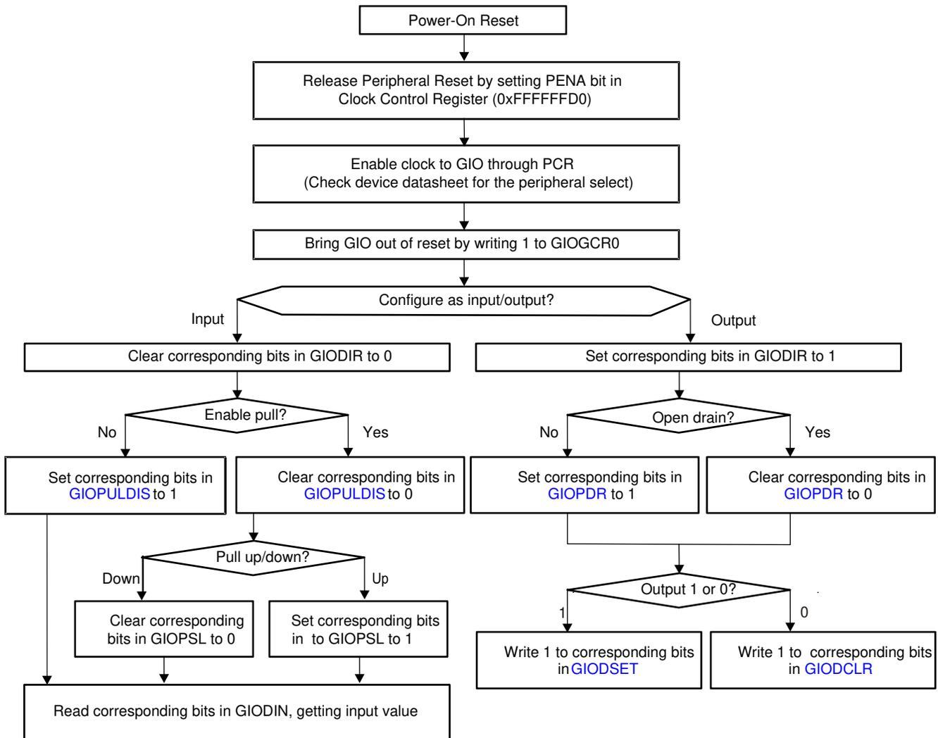
**Figure 17-1. I/O Function Quick Start Flow Chart**
