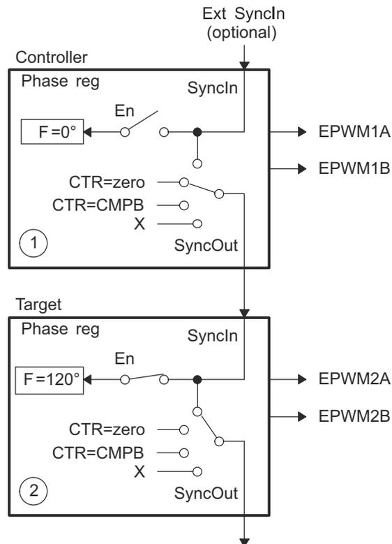
**Figure 18-61. Configuring Two PWM Modules for Phase Control**
