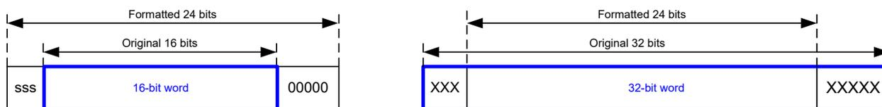
For 16-bit case, if SRC\_SCAL = 3, then 5 zeros are padded at the LSB, and 3 redundant (extension) bits are padded at the MSB
