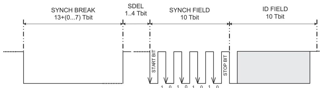
**Figure 19-14. Message Header in Terms of  $T_{\text{bit}}$**
