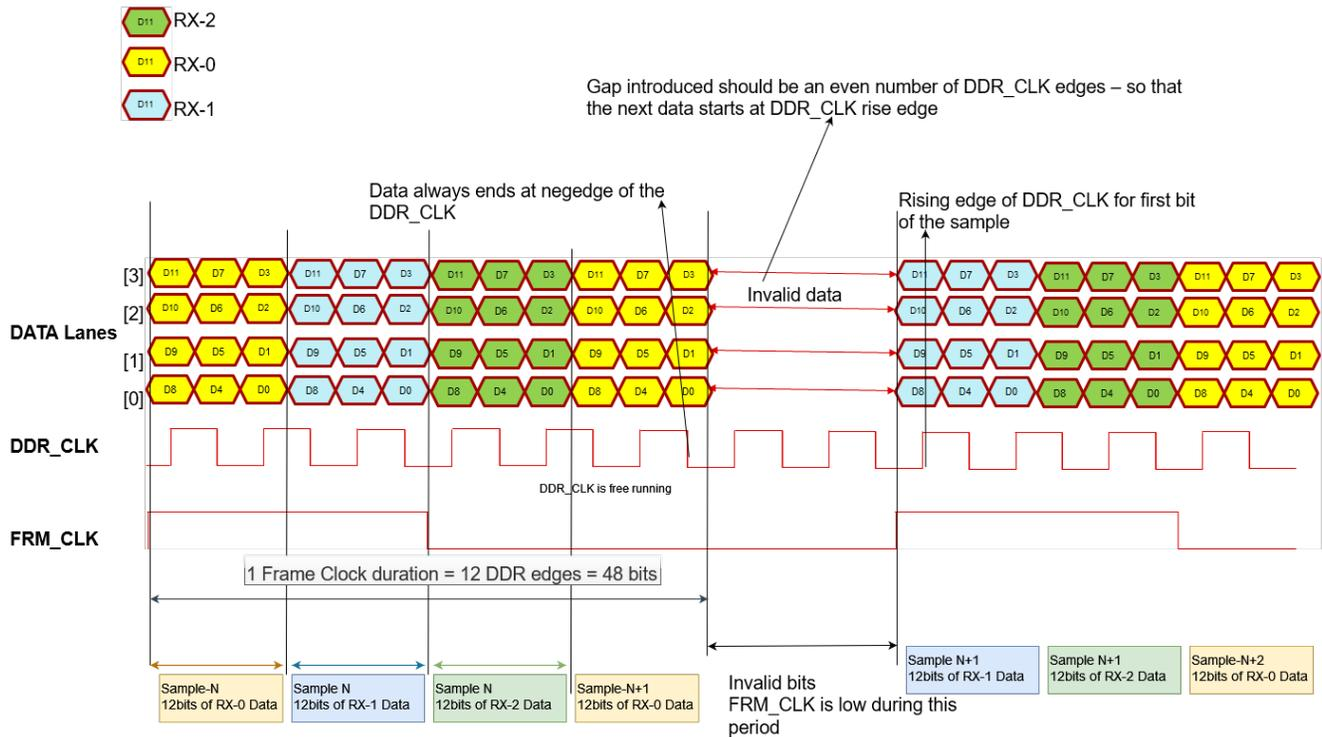
The following are the data format requirements which are shown in the diagram above and the excel sheet below.
