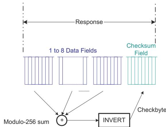
Figure 19-21. Classic Checksum Generation at Transmitting Node
