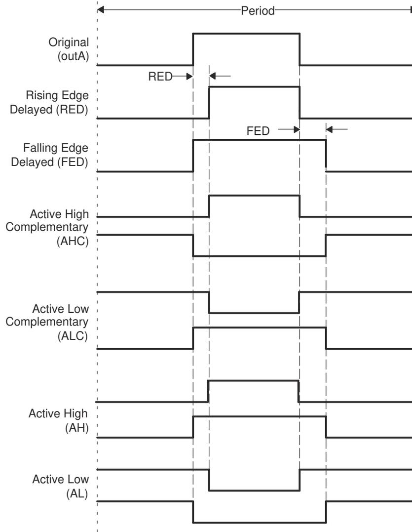
Figure 18-29. Dead-Band Waveforms for Typical Cases (0% < Duty < 100%)
