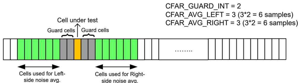
**Figure 10-26. CFAR-CA: Cells used for Surrounding Noise Average**
