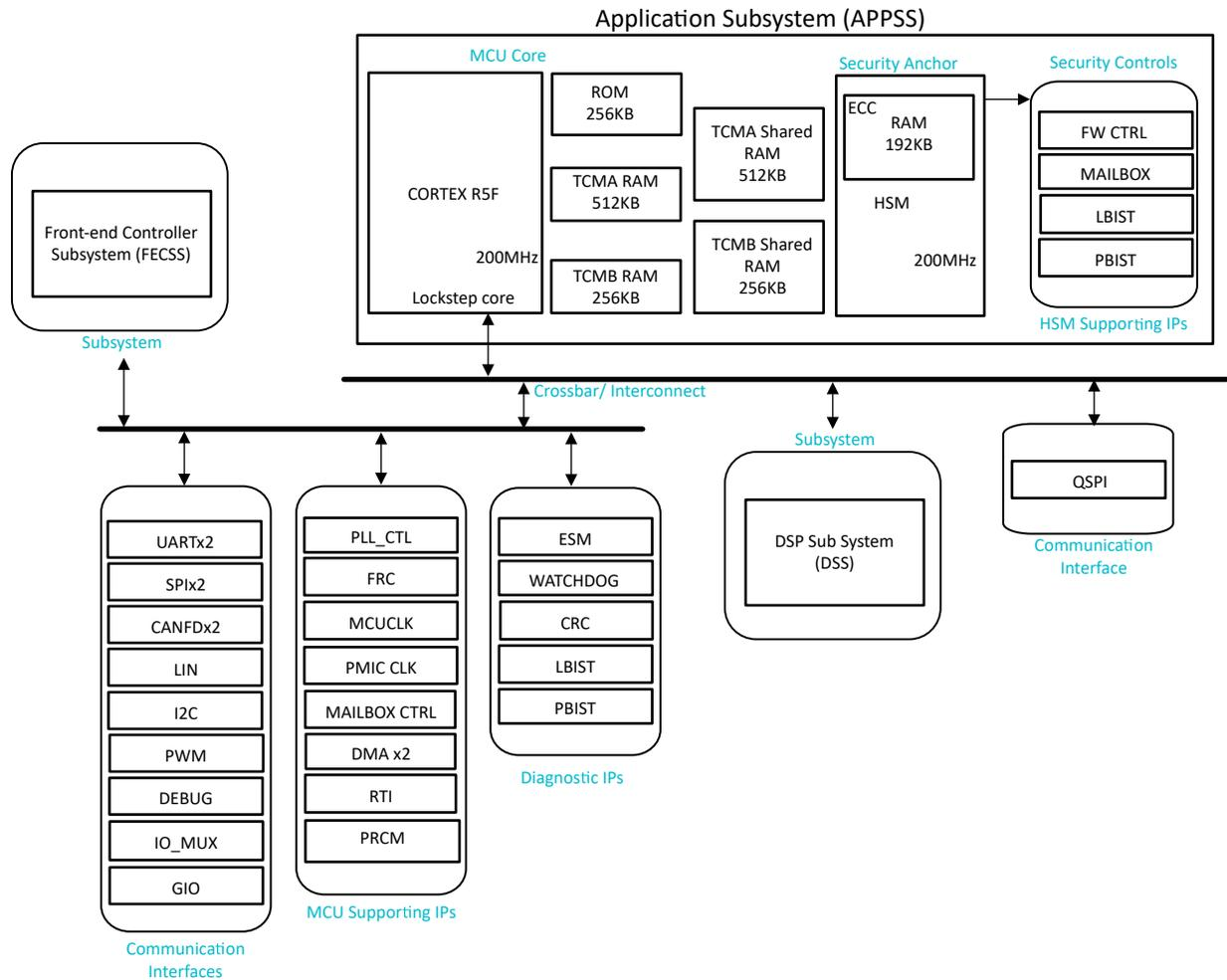
Figure 3-1. Application Subsystem Infrastructure
