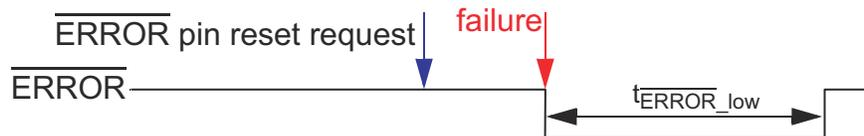
Figure 22-15.  $\overline{\text{ERROR}}$  Pin Timing - Example 5
