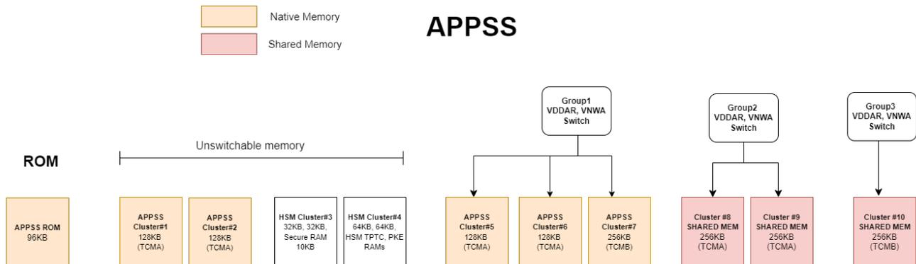
Referring to the diagram above "Memory Cluster Diagram", there are 10 memory clusters in APPSS sub system, divided in 4 groups (unswitchable, group 1-3). Each of the memory clusters can be configured to be power up or power down separately in domains power up or down state.
