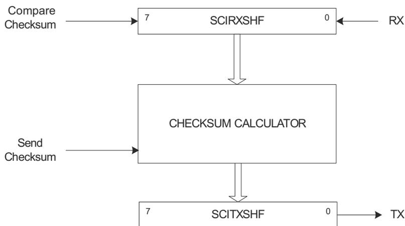
**Figure 19-19. Checksum Compare and Send for Extended Frames**
