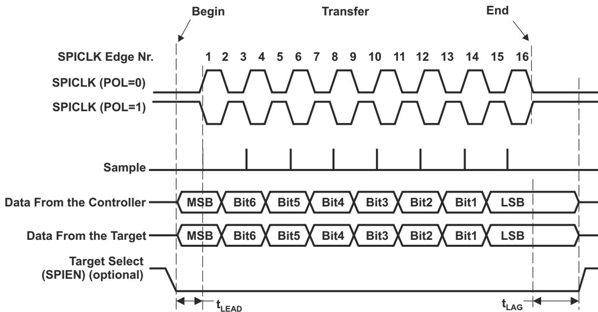
Figure 13-7. Full Duplex Single Transfer Format with PHA = 0
