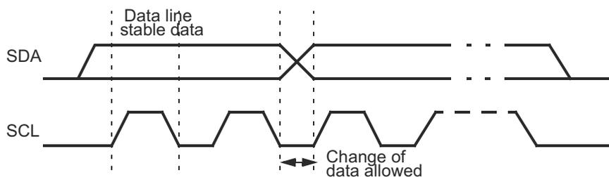
Figure 16-4. Bit Transfer on the I2C Bus
