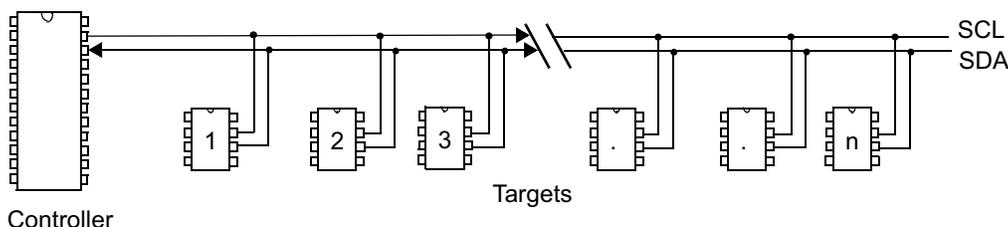
**Figure 16-1. Multiple I2C Modules Connection Diagram**
