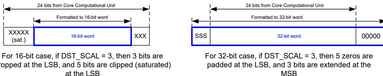
**Figure 10-11. Output Formatter Data Scaling**
