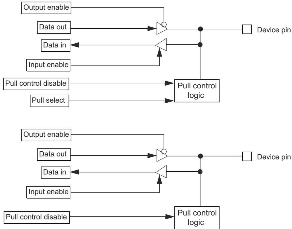
**Figure 15-8. GPIO Functionality**
