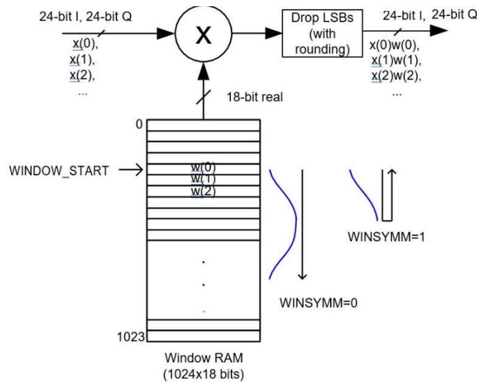
**Figure 10-14. Windowing Computation**
