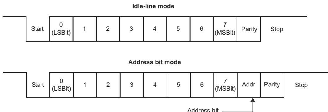
**Figure 19-3. Typical SCI Data Frame Formats**
