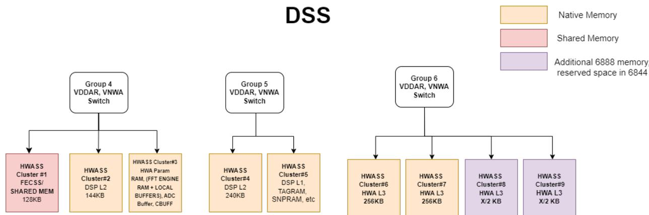
The DSS sub system can be taken powered down independently of the APPSS and FECSS. R5 can force power down or power up of DSS domain. Referring to the diagram above "Memory Cluster Diagram", there are 7 memory clusters in DSS sub system. Each of the memory clusters can be configured to be power up or power down separately in domains power up or down state. The DSS sub system can be configured in one of the following three states:
