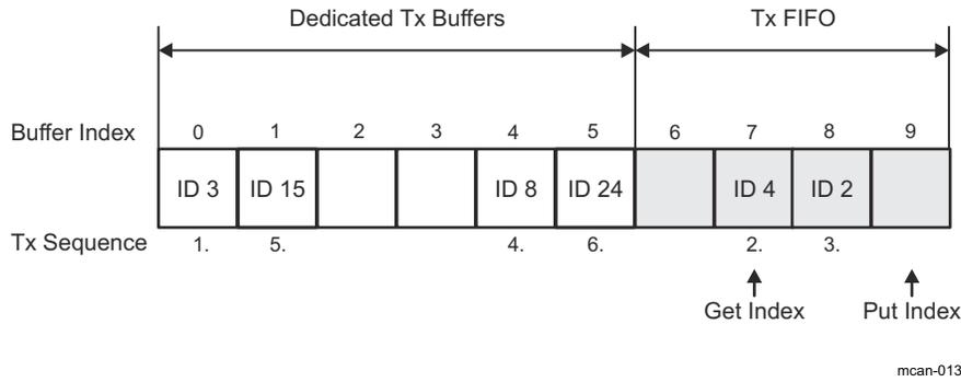
Figure 12-12. Mixed Dedicated Tx Buffers /Tx FIFO (example)
