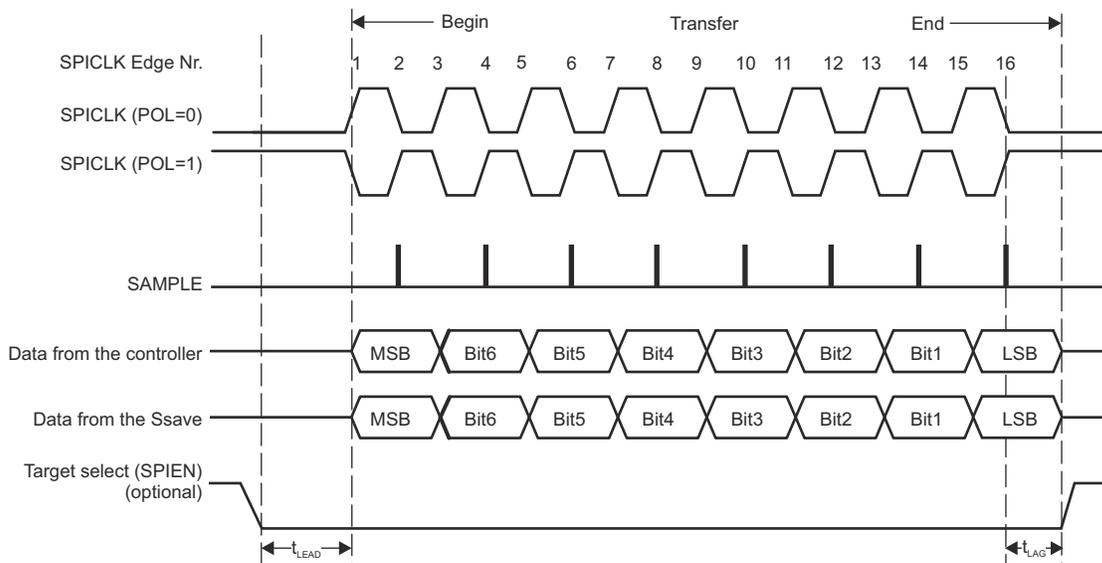
**Figure 13-8. Full Duplex Single Transfer Format With PHA = 1**
