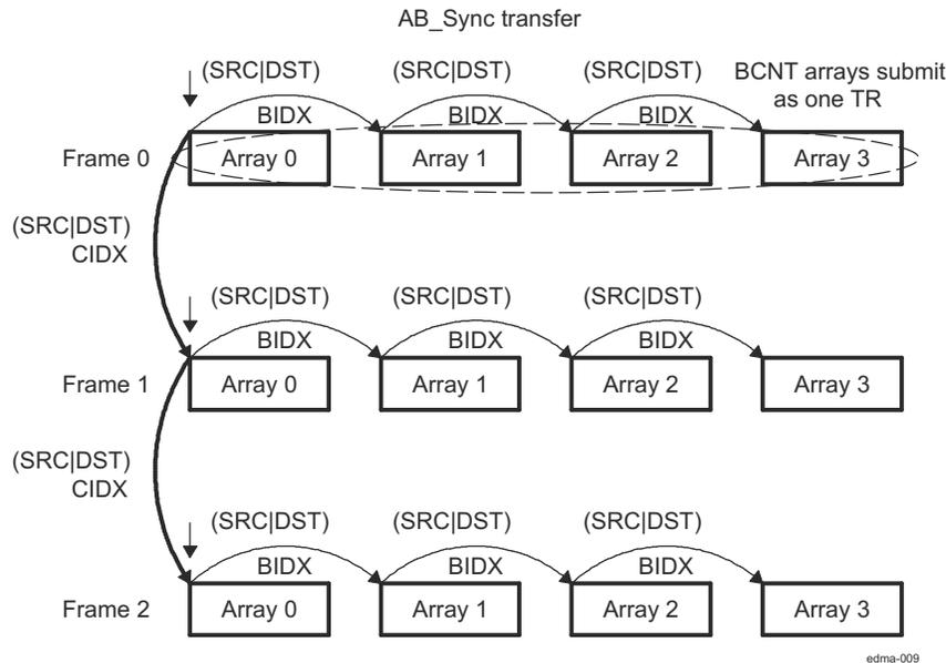
**Figure 11-7. AB-Synchronized Transfers (ACNT = n, BCNT = 4, CCNT = 3)**
