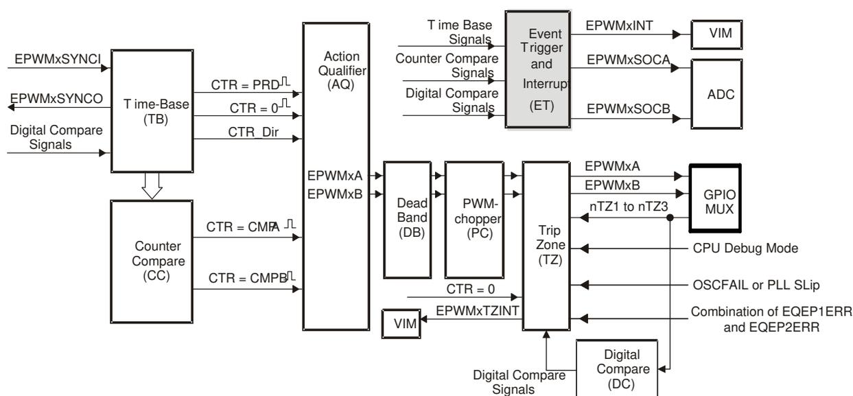
**Figure 18-38. Event-Trigger Submodule**
