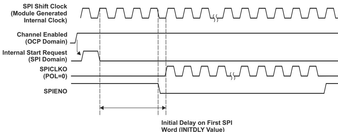
**Figure 13-21. Controller Single Channel Initial Delay**
