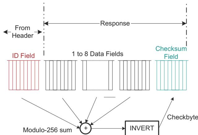
Figure 19-22. LIN 2.0-Compliant Checksum Generation at Transmitting Node
