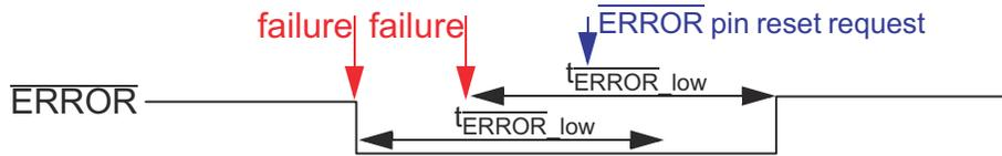
Figure 22-14.  $\overline{\text{ERROR}}$  Pin Timing - Example 4
