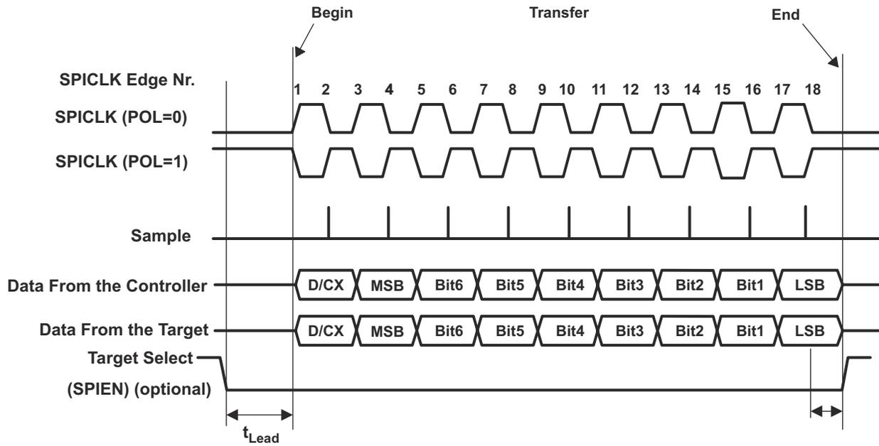
Figure 13-11. Extended SPI Transfer With Start Bit PHA = 1
