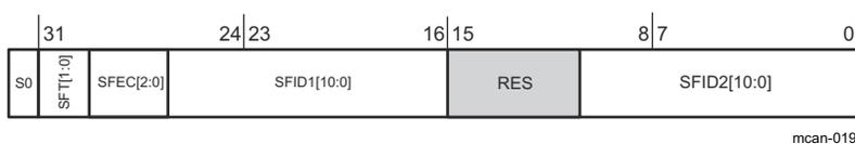
**Figure 12-18. Standard Message ID Filter Element Structure**
