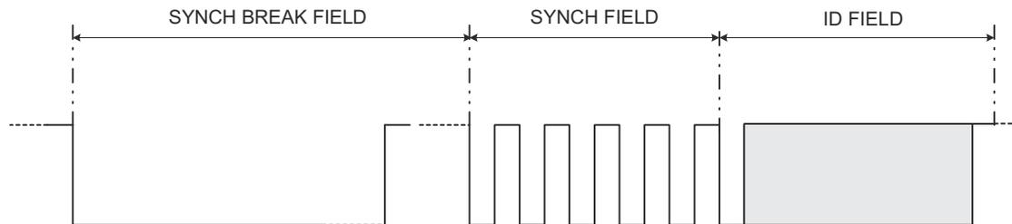
**Figure 19-12. Header 3 Fields: Synch Break, Synch, and ID**
