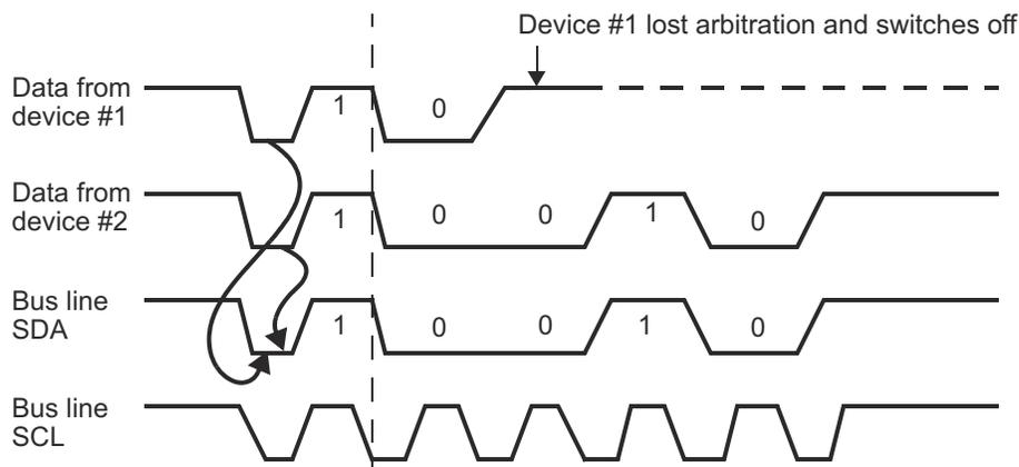
**Figure 16-11. Arbitration Procedure Between Two Controller Transmitters**
