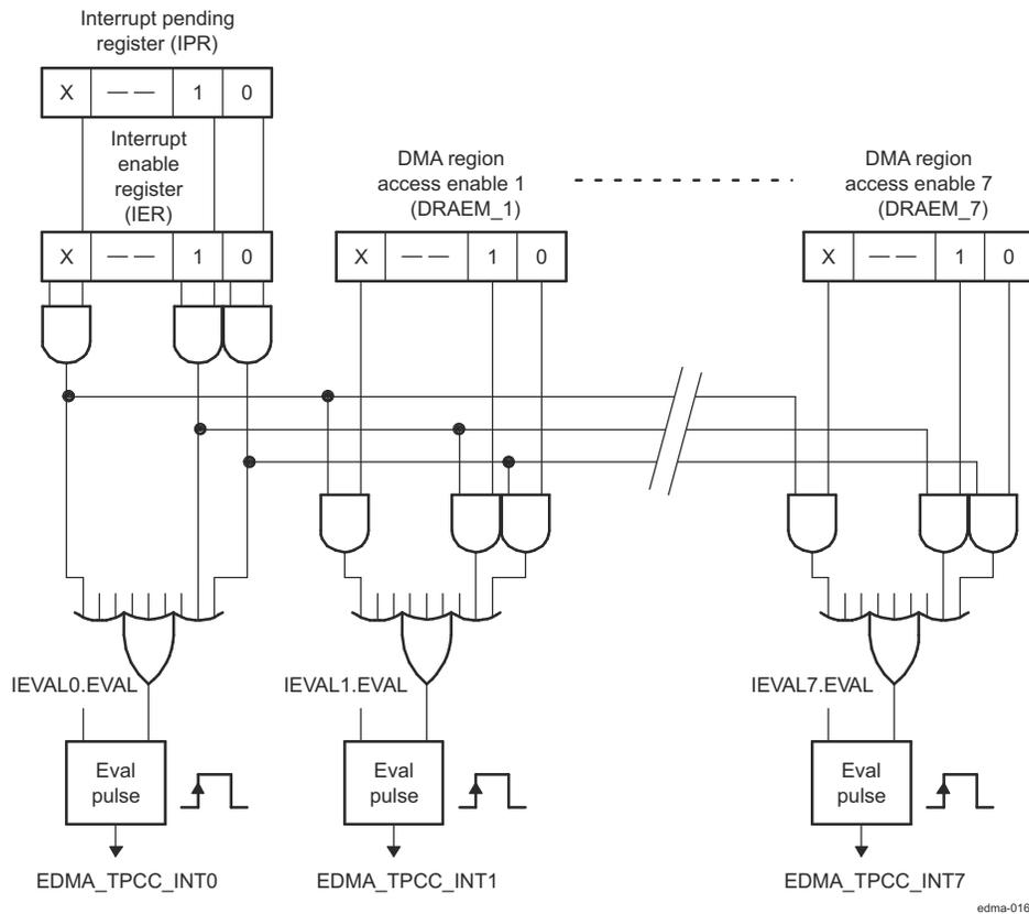
Figure 11-14. Interrupt Diagram
