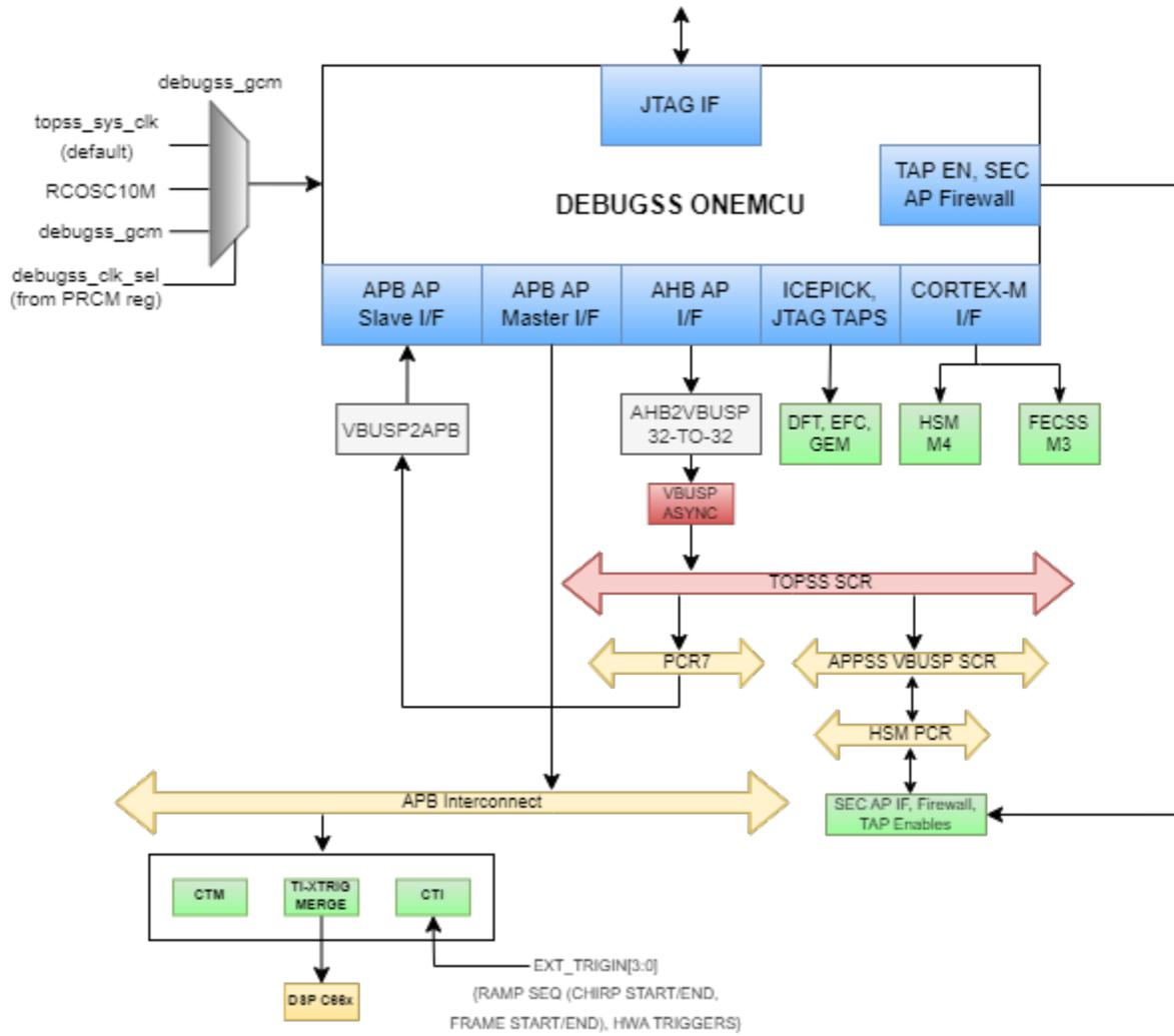
Figure 21-2. Onemcu DebugSS Integration
