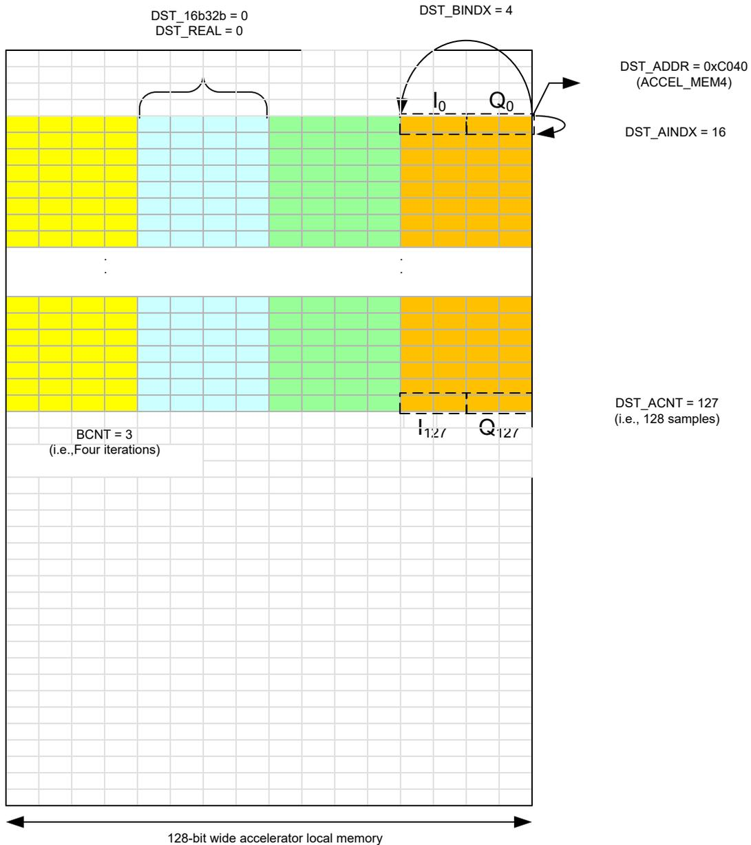
**Figure 10-10. Output Formatter Destination Memory Access Pattern (Example)**
