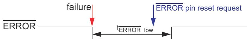
Figure 22-12.  $\overline{\text{ERROR}}$  Pin Timing - Example 2
