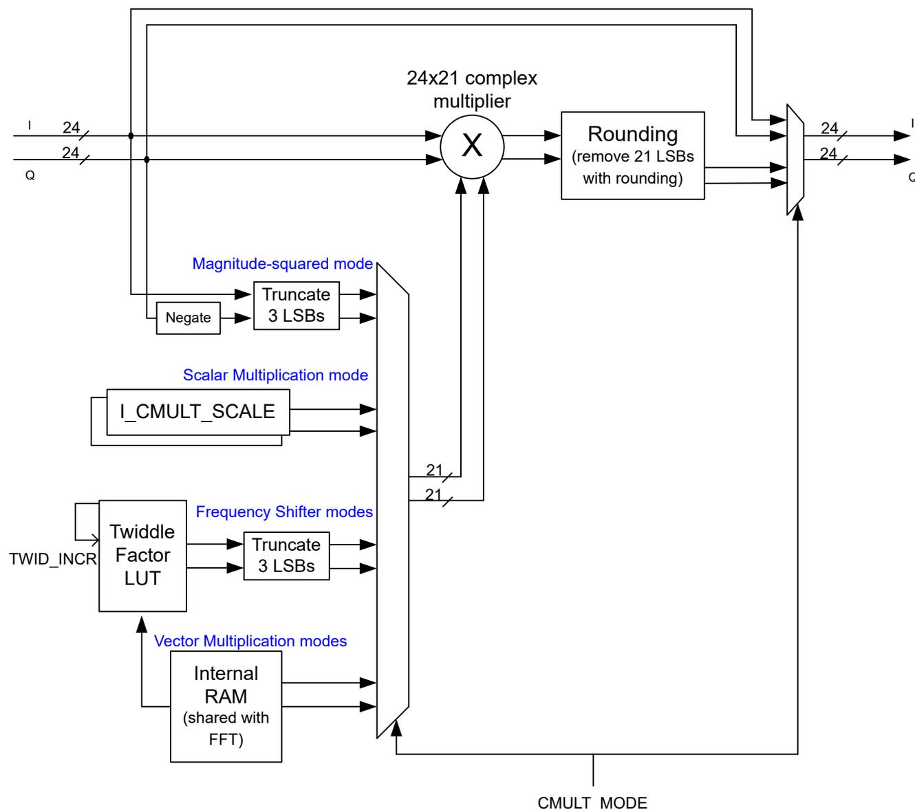
Figure 10-22. Complex multiplication capability in Pre-processing block
