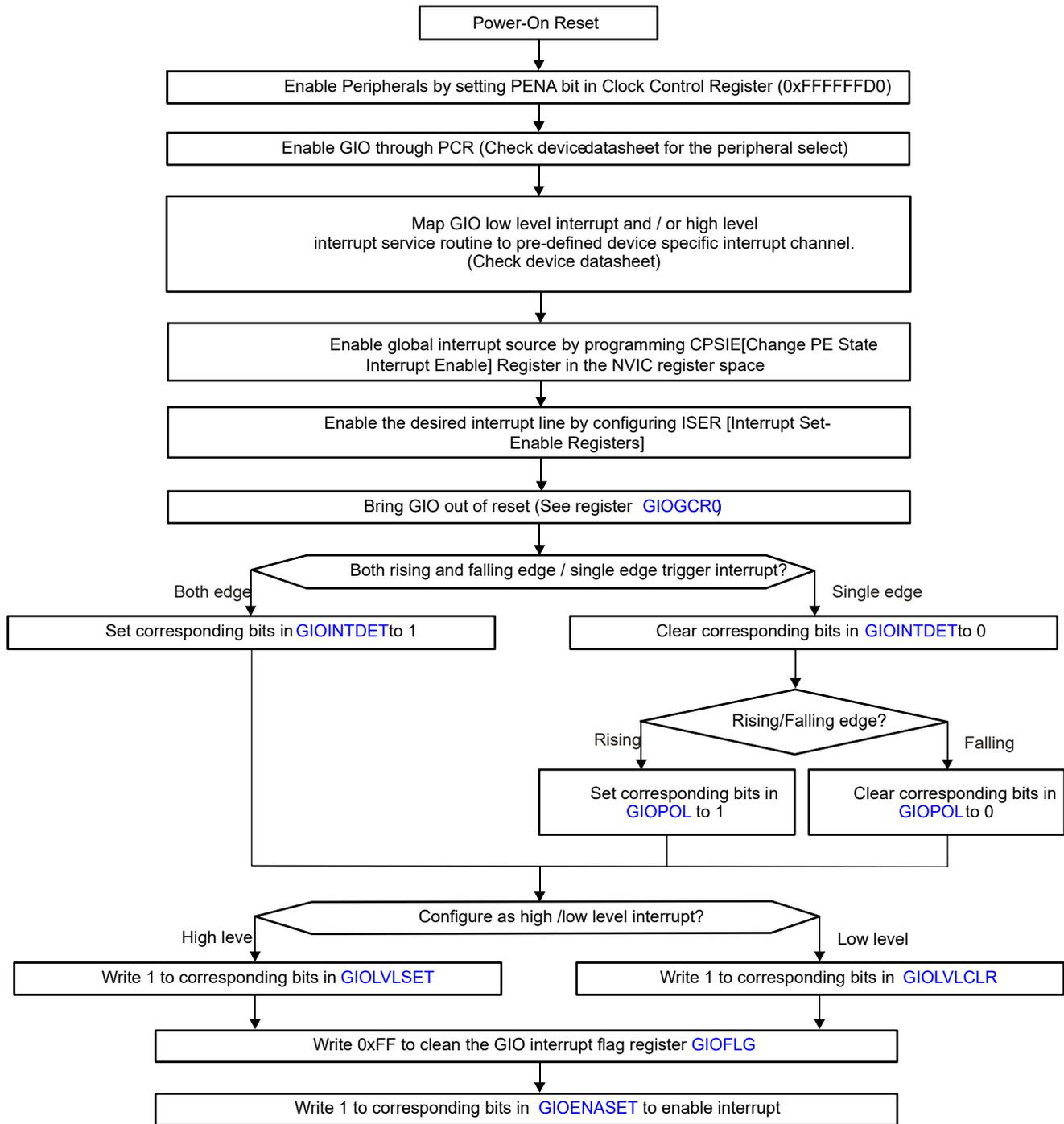
Figure 17-2. Interrupt Generation Function Quick Start Flow Chart
