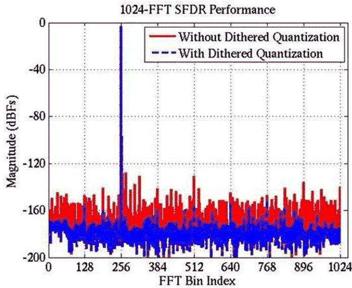
Figure 10-16. FFT SFDR Performance with and Without Dithering
