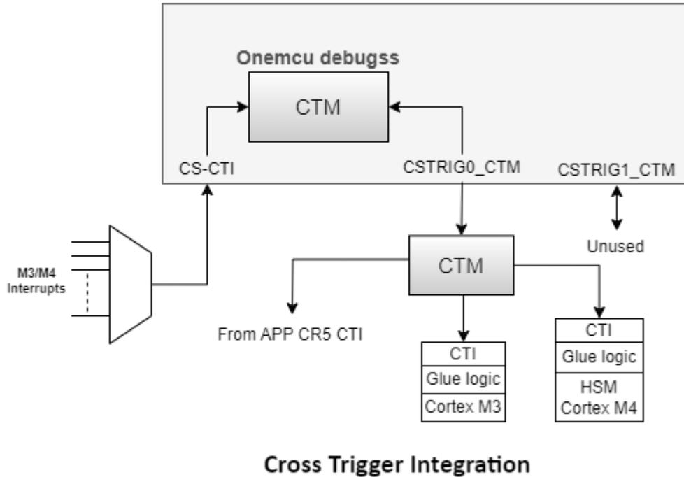
Figure 21-3. Cross Trigger Integration
