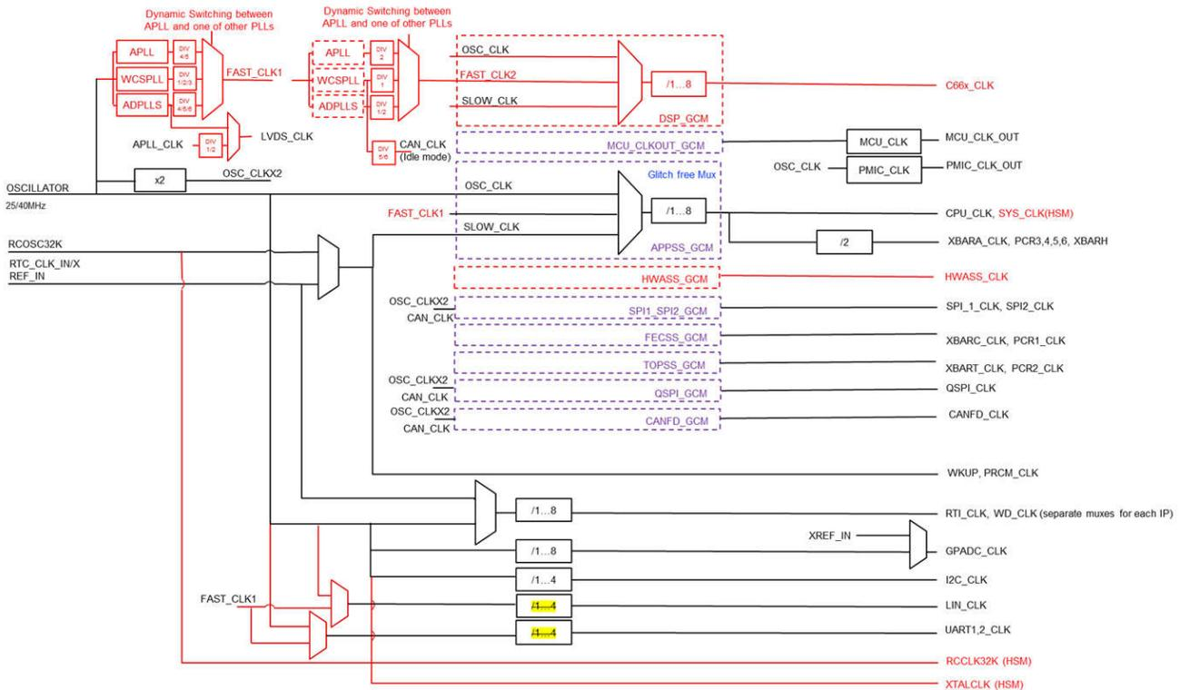
Figure 5-2. Clock Tree Configuration
