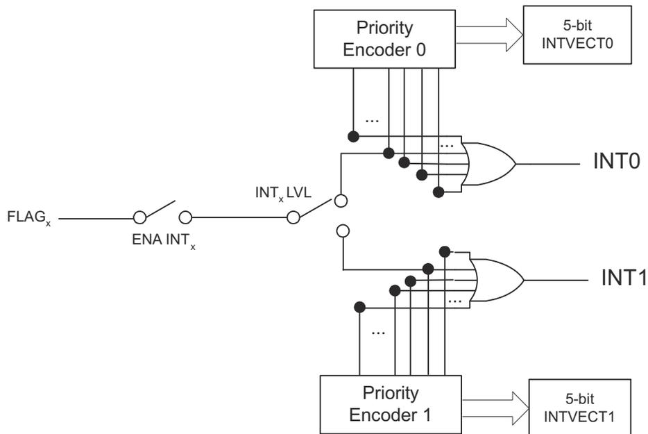
**Figure 19-10. Interrupt Generation for Given Flags**
