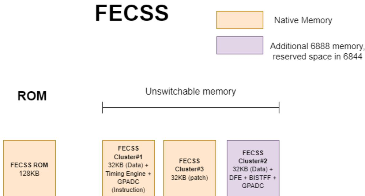
The FECSS sub system can be taken powered down independently of the APPSS and DSS. R5 can force power down or power up of FECSS domain. Referring to the diagram above "Memory Cluster Diagram", there are three memory clusters in FECSS sub system. Each of the memory clusters can be configured to be power up or power down separately in domains power up or down state. The FECSS sub system can configured in one of the following three states,
