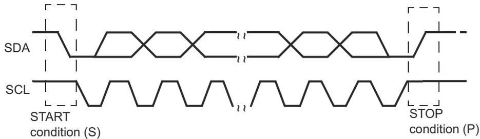
Figure 16-5. I2C Module START and STOP Conditions
