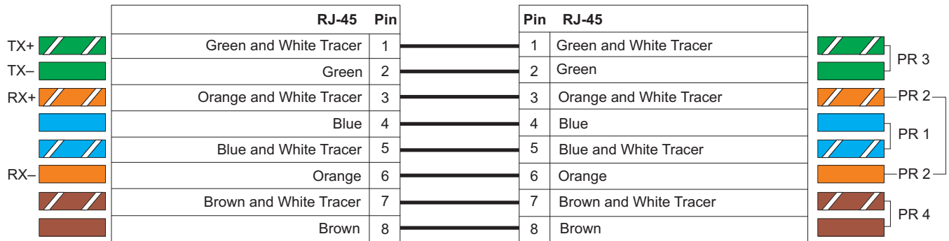
Figure 7. RJ-45 Cable Details
