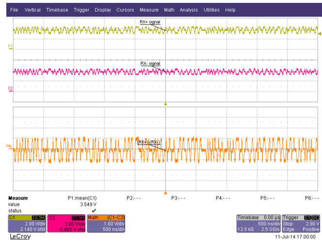
Figure 23. RX+ and RX– Signals
