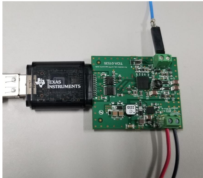
Figure 7. SM-USB-DIG Connected to TIDA-01535
