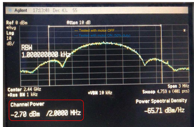
Figure 39. Measured TX Channel Power Measurement at 2440 MHz, 0-dBm Level With Motor ON and OFF
