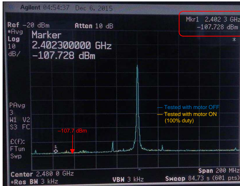
Figure 42. TX Performance With Bluetooth Channel Frequency of 2480 MHz
