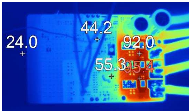
Figure 27. Thermal Image at 18-V DC Input, 25.6-A RMS Winding Current, 100% Duty Cycle
