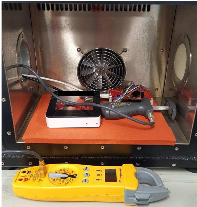
Figure 43. Test Setup of Temperature Chamber System
