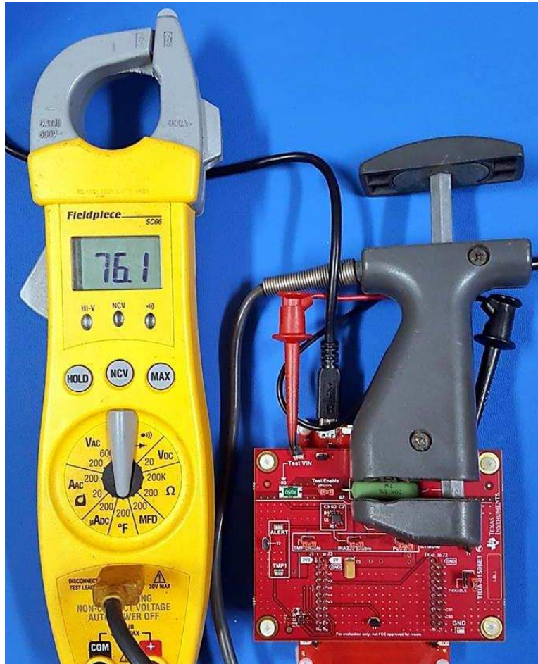
Figure 41. Test Setup of Ambient Load Temperature
