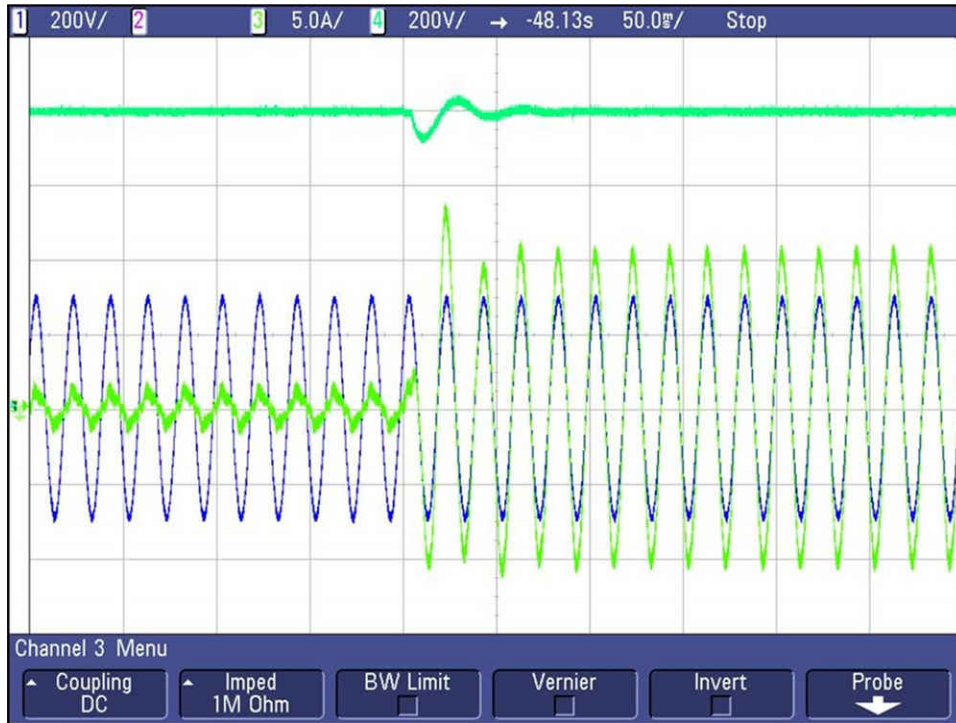
Figure 3-43. Voltage Step - 400 W → 4.4 kW
