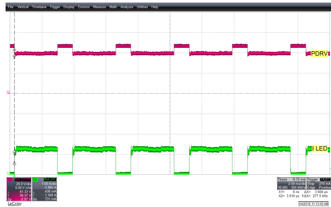
Figure 12. 240 Hz, 33% Duty Cycle PWM Dimming Feature with R18 (100 K \Omega )—CH1: PDRV, and CH4: LED Current
