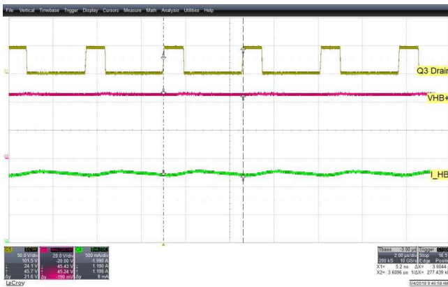
Figure 11. Normal Operation Fswitch at 275 KHz—CH1: Switch Node (Q3 Drain), CH2: VLED in High Beam and Low Beam Mode, and CH4: LED Current for Output power of 55 W
