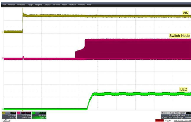
Figure 9. Low Beam Mode Startup—CH1: VIN, CH2: Switch Node (Q3 Drain) Voltage, and CH4: LED Current
