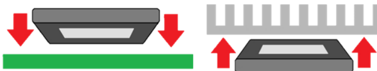
Figure 2-2. Pad-Down vs. Pad-Up Audio Amplifier
