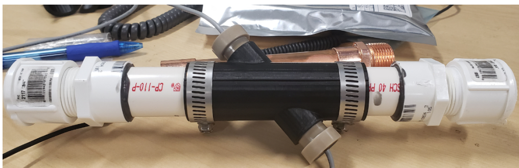
Figure 1-3. 3D Printed Fixture Attached the PVC Pipe
