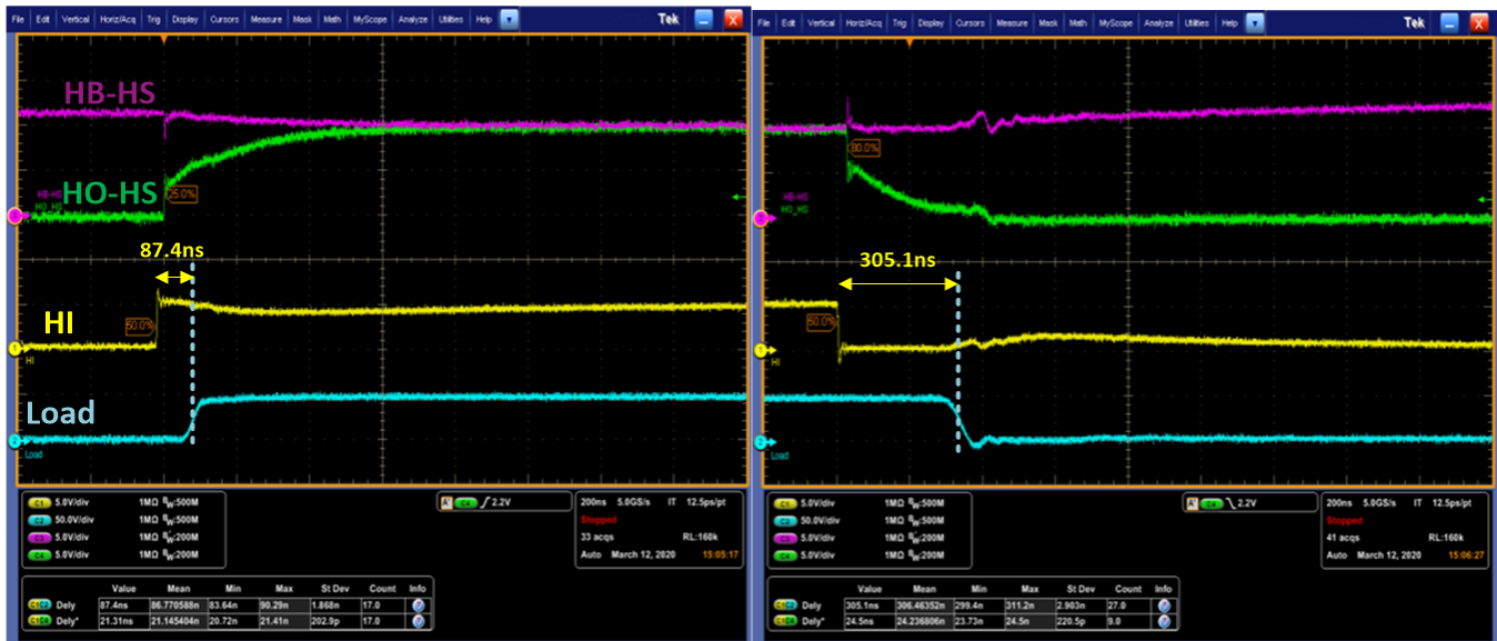
Figure 8. Response Time of the Bidirectional Switch Driver UCC27284
