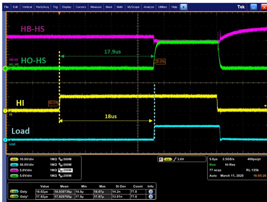
Figure 10. Response Time of the Bidirectional Switch Driver
