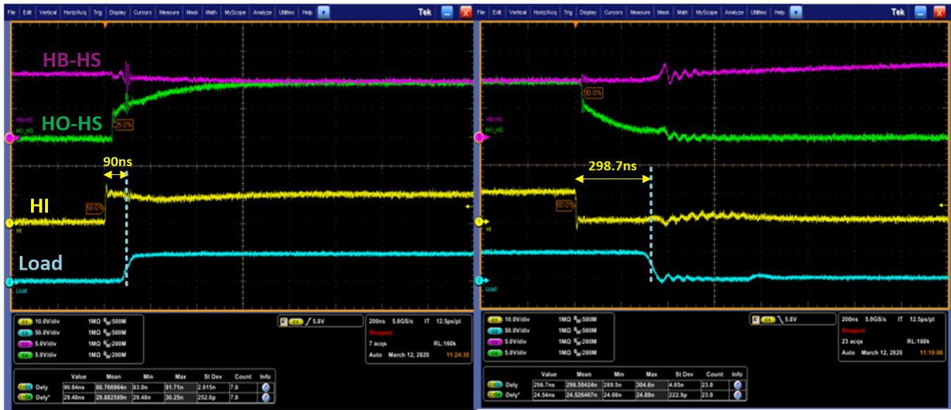
Figure 7. Response Time of the Bidirectional Switch Driver UCC27212-Q1
