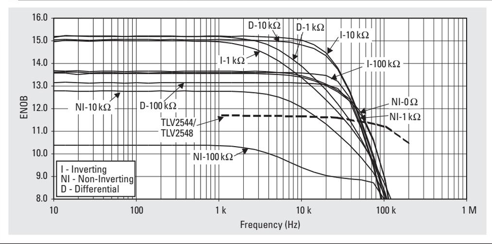
**Figure 5. The TLV2772 at 3.3 V**
