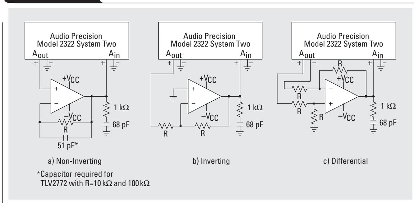
\*Capacitor required for TLV2772 with R=10 kΩ and 100 kΩ
